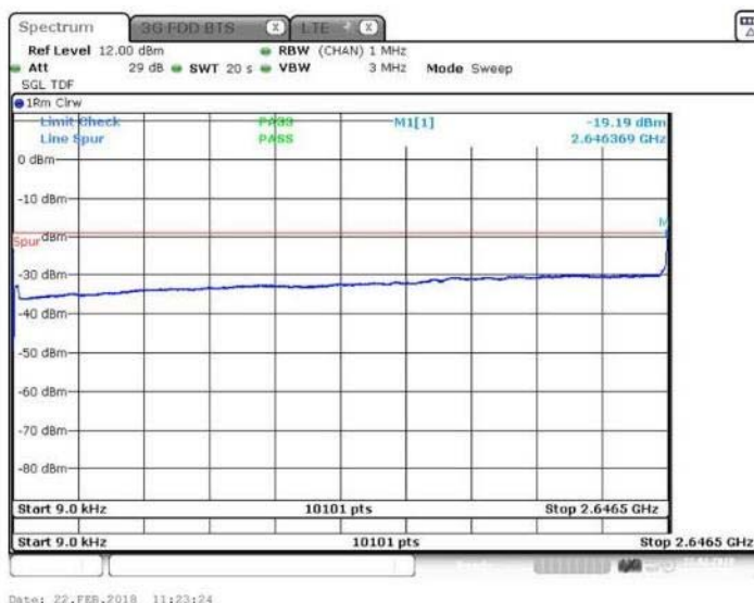
Figure 113 Spurious Emissions (9kHz – 2.6465 GHz) – 256QAM (2655 MHz, 15 MHz Channel BW)
