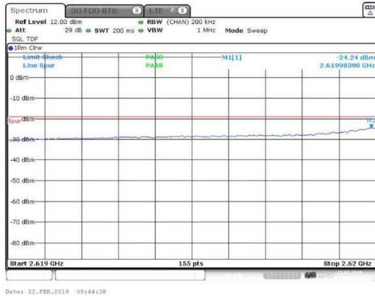
Figure 105 Spurious Emissions (Lower Band Edge) – 64QAM (2627.5 MHz, 15 MHz Channel BW)
