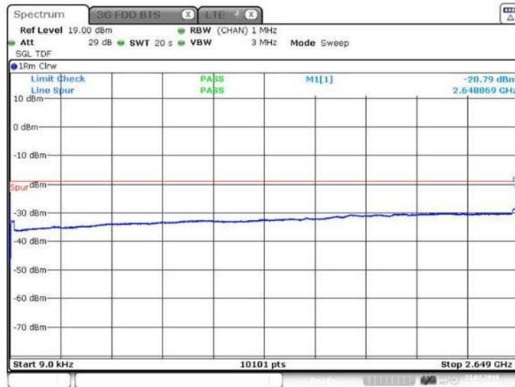
Figure 71 Spurious Emissions (9kHz – 2.649 GHz) – QPSK (2655 MHz, 10 MHz Channel BW)
