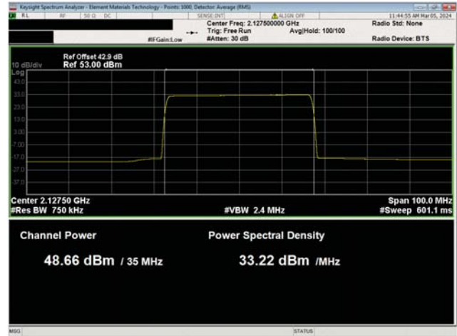
Band n66, 5G NR, 2110.0 MHz - 2200.0 MHz 35 MHz Channel Bandwidth 256QAM Modulation Low Channel, 2127.5 MHz
