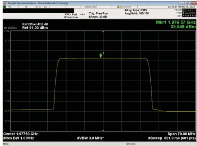
Band n25, 5G NR, 1930.0 MHz - 1995.0 MHz 35 MHz Channel Bandwidth 256QAM Modulation High Channel, 1977.5 MHz
