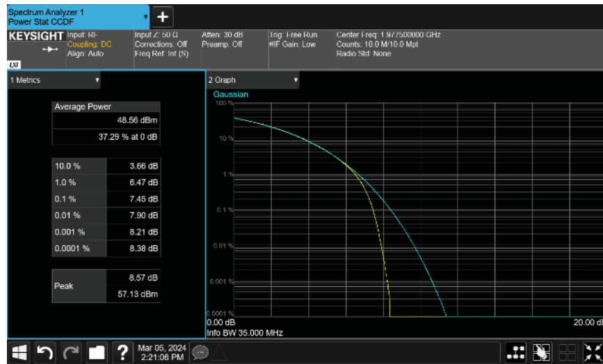
Band n25, 5G NR, 1930.0 MHz - 1995.0 MHz 35 MHz Channel Bandwidth 256QAM Modulation High Channel, 1977.5 MHz
