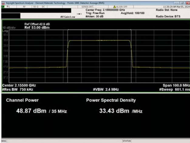
Band n66, 5G NR, 2110.0 MHz - 2200.0 MHz 35 MHz Channel Bandwidth 64QAM Modulation Mid Channel, 2155.0 MHz
