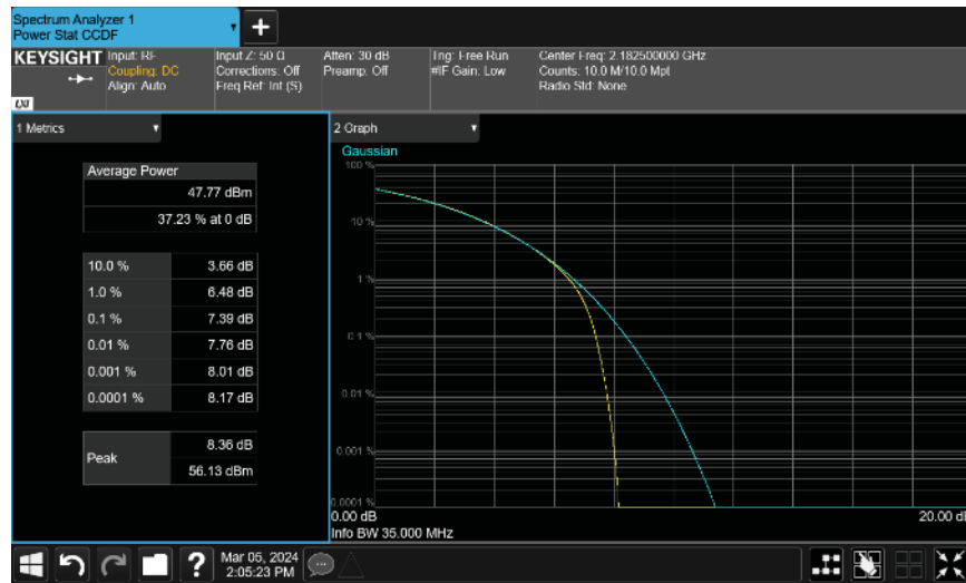
Band n66, 5G NR, 2110.0 MHz - 2200.0 MHz 35 MHz Channel Bandwidth 256QAM Modulation High Channel, 2182.5 MHz
