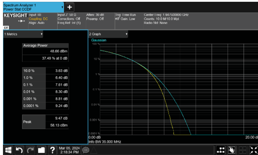
Band n25, 5G NR, 1930.0 MHz - 1995.0 MHz 35 MHz Channel Bandwidth 256QAM Modulation Low Channel, 1947.5 MHz
