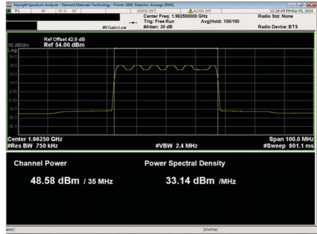
Band n25, 5G NR, 1930.0 MHz - 1995.0 MHz 35 MHz Channel Bandwidth 16QAM Modulation Mid Channel, 1962.5 MHz
