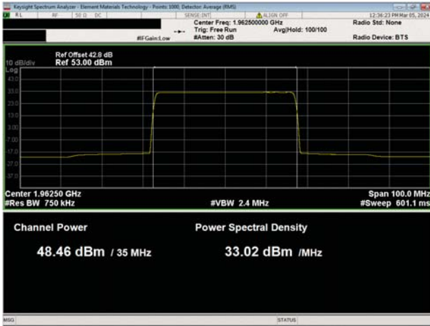
Band n25, 5G NR, 1930.0 MHz - 1995.0 MHz 35 MHz Channel Bandwidth 256QAM Modulation Mid Channel, 1962.5 MHz
