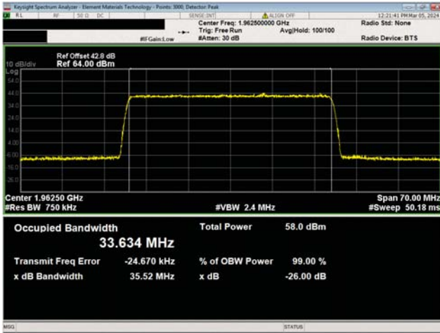
Band n25, 5G NR, 1930.0 MHz - 1995.0 MHz 35 MHz Channel Bandwidth QPSK Modulation Mid Channel, 1962.5 MHz
