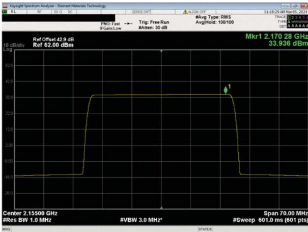
Band n66, 5G NR, 2110.0 MHz - 2200.0 MHz 35 MHz Channel Bandwidth QPSK Modulation Mid Channel, 2155.0 MHz
