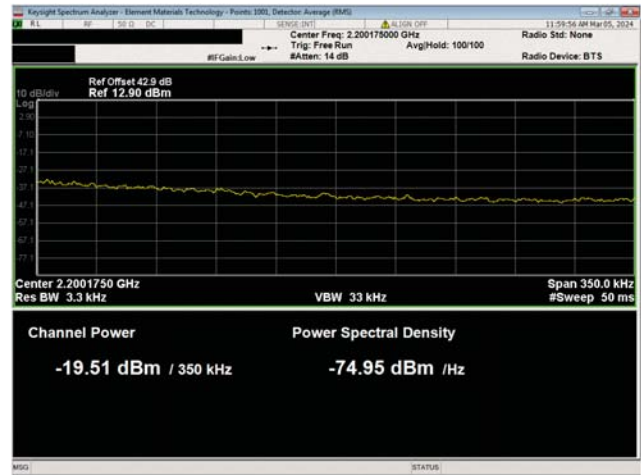
Band n66, 5G NR, 2110.0 MHz - 2200.0 MHz 35 MHz Channel Bandwidth 256QAM Modulation High Channel, 2182.5 MHz
