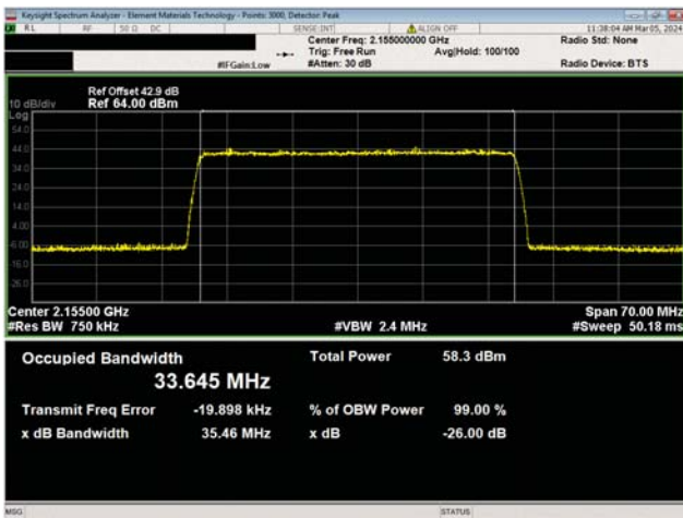
Band n66, 5G NR, 2110.0 MHz - 2200.0 MHz 35 MHz Channel Bandwidth 256QAM Modulation Mid Channel, 2155.0 MHz
