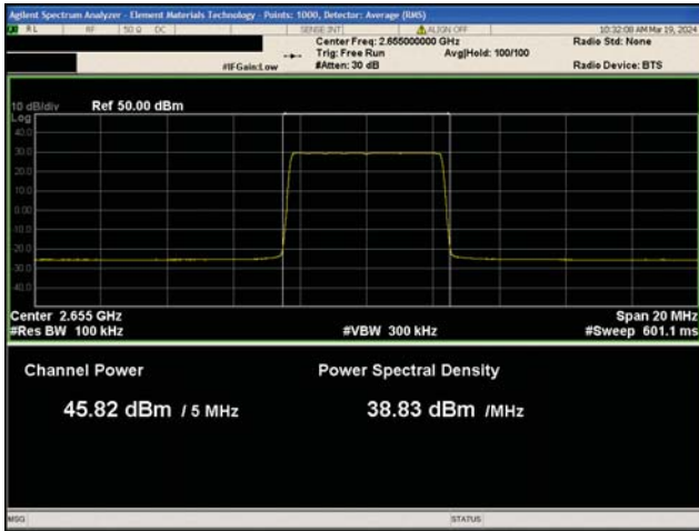
2G GSM/EDGE PCS Band 2 Test Case 1 LTE5 QPSK Modulation Mid Channel, 2655.0 MHz
