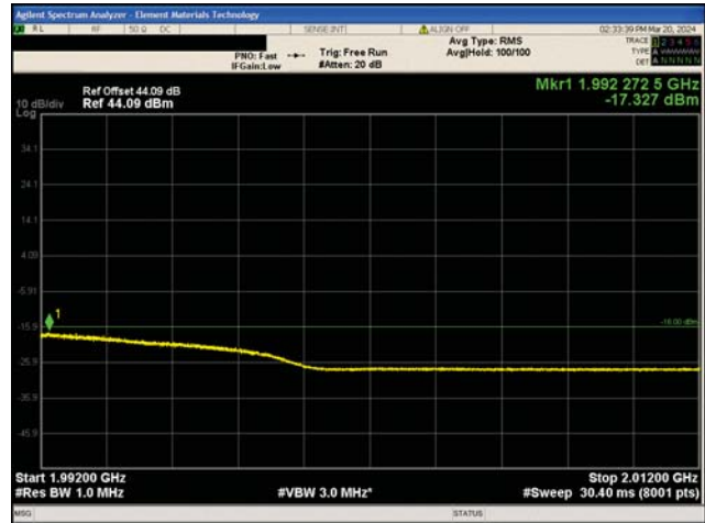
3G WCDMA PCS Band II Test Case 1 QPSK Modulation High Channel, 1987.6 MHz
