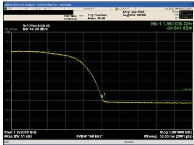
3G WCDMA PCS Band II Test Case 1 64QAM Modulation High Channel, 1987.6 MHz
