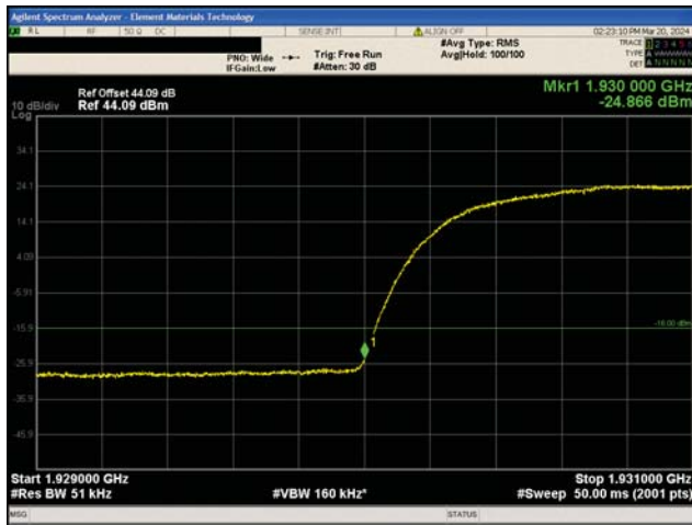
3G WCDMA PCS Band II Test Case 1 16QAM Modulation Low Channel, 1932.4 MHz
