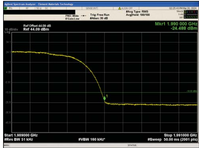
3G WCDMA PCS Band II Test Case 1 16QAM Modulation High Channel, 1987.6 MHz
