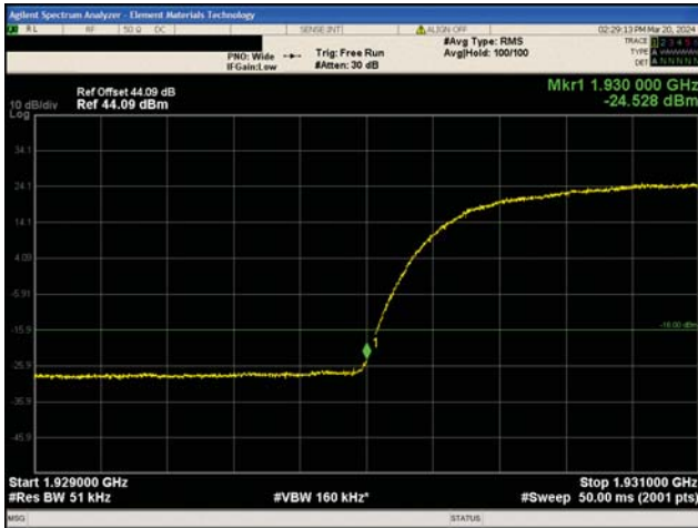
3G WCDMA PCS Band II Test Case 1 QPSK Modulation Low Channel, 1932.4 MHz
