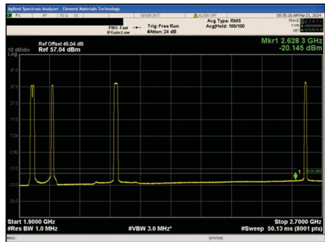
3G WCDMA PCS Band II Test Case 1 64QAM Modulation (WCDMA) and QPSK Modulation (LTE)
