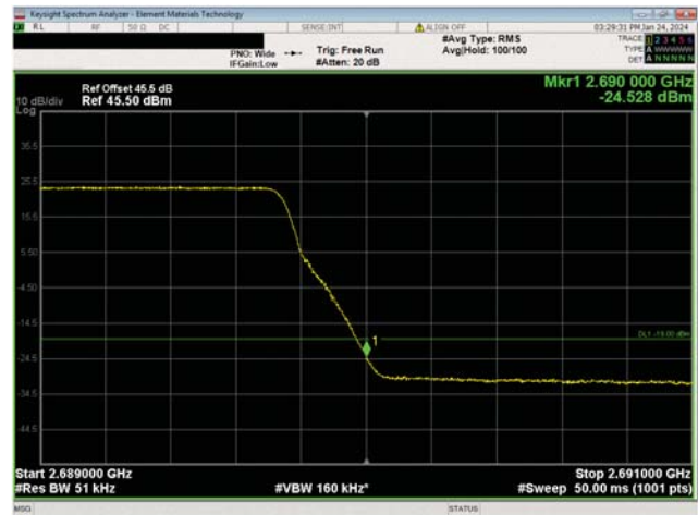
BRS Multicarrier Multiband Test Case 1 QPSK Modulation BRS n7, NR5, High Ch, 2687.5 MHz
