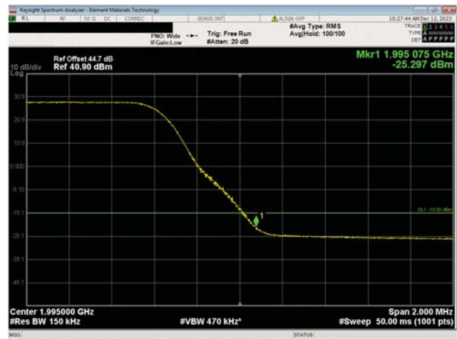
PCS Band n25, 1930 MHz - 1995 MHz 15 MHz Bandwidth 256QAM Modulation High Ch, 1987.5 MHz
