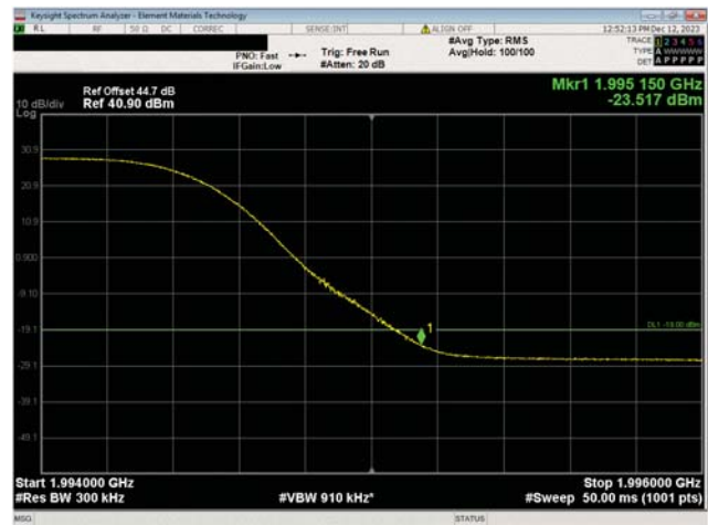
PCS Band n25, 1930 MHz - 1995 MHz 30 MHz Bandwidth 256QAM Modulation High Ch, 1980.0 MHz
