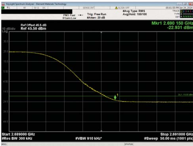
BRS Multicarrier Multiband Test Case 3 QPSK Modulation BRS n7, NR30, High Ch, 2645.0 MHz
