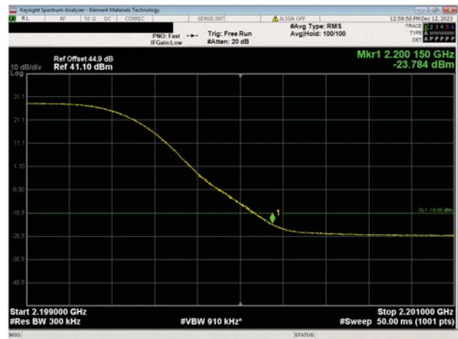
AWS Band n66, 2110 MHz - 2200 MHz 30 MHz Bandwidth 256QAM Modulation High Ch, 2185.0 MHz
