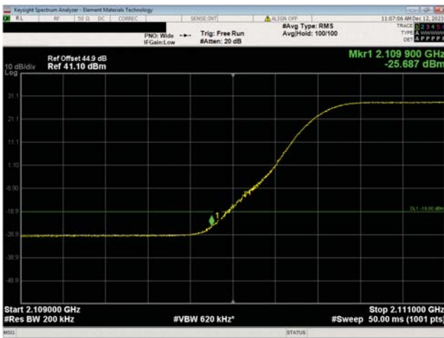
AWS Band n66, 2110 MHz - 2200 MHz 20 MHz Bandwidth 256QAM Modulation Low Ch, 2120.0 MHz
