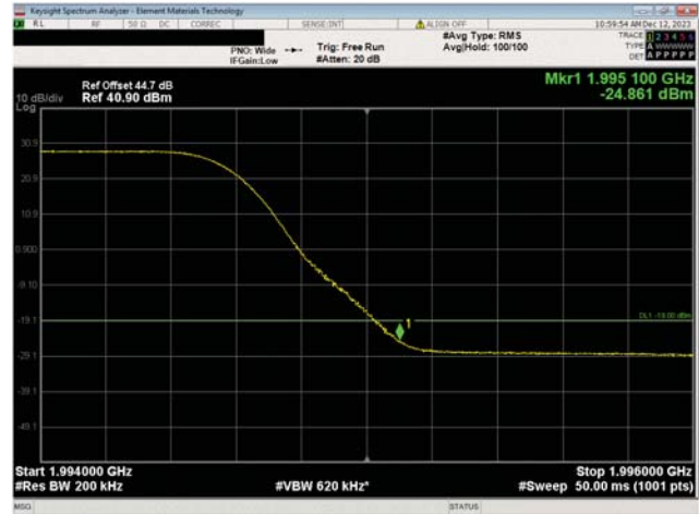
PCS Band n25, 1930 MHz - 1995 MHz 20 MHz Bandwidth 256QAM Modulation High Ch, 1985.0 MHz
