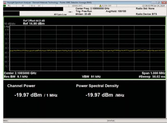
AWS Multicarrier Multiband Test Case 1 QPSK Modulation AWS n66, NR5, Low Ch, 2112.5 MHz
