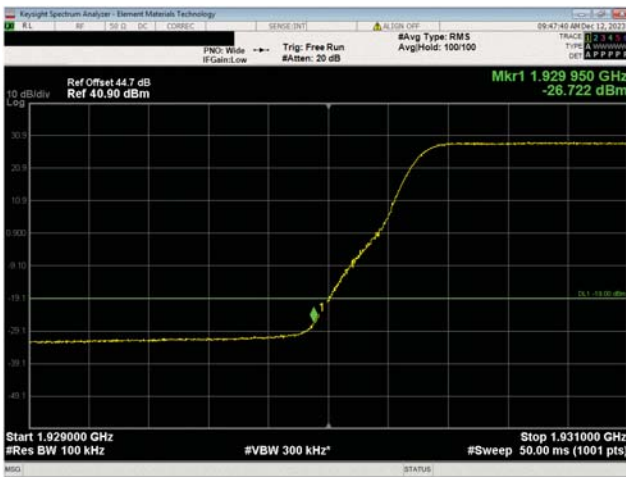
PCS Band n25, 1930 MHz - 1995 MHz 10 MHz Bandwidth 256QAM Modulation Low Ch, 1935.0 MHz
