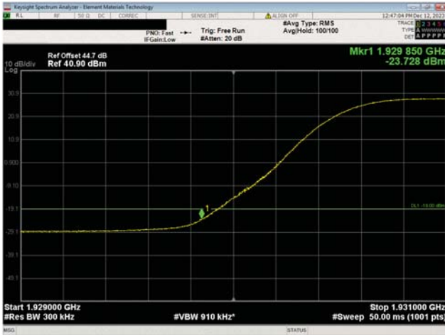
PCS Band n25, 1930 MHz - 1995 MHz 30 MHz Bandwidth 256QAM Modulation Low Ch, 1945.0 MHz
