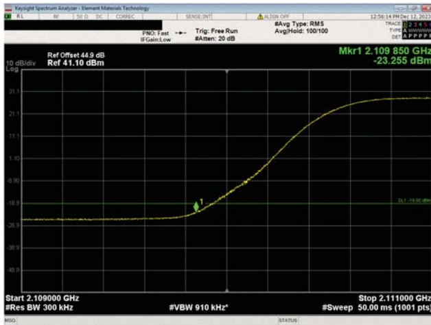
AWS Band n66, 2110 MHz - 2200 MHz 30 MHz Bandwidth 256QAM Modulation Low Ch, 2125.0 MHz
