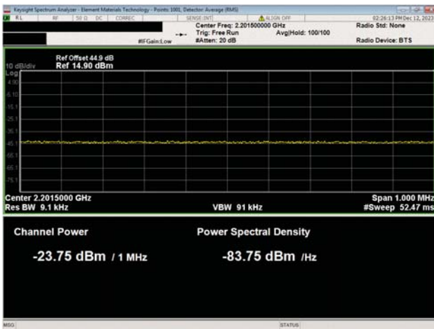
AWS Band n66, 2110 MHz - 2200 MHz 40 MHz Bandwidth 256QAM Modulation High Ch, 2180.0 MHz
