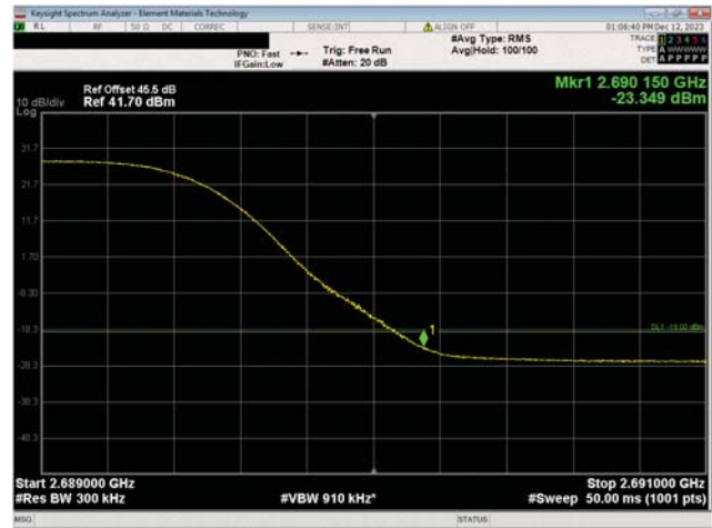
BRS Band n7, 2620 MHz - 2690 MHz 30 MHz Bandwidth 256QAM Modulation High Ch, 2675.0 MHz
