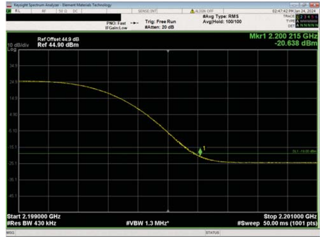
AWS Multicarrier Multiband Test Case 3 QPSK Modulation AWS n66, NR40, High Ch, 2140.0 MHz
