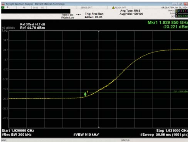
PCS Multicarrier Multiband Test Case 2 QPSK Modulation PCS n25, NR30, Low Ch, 1945.0 MHz
