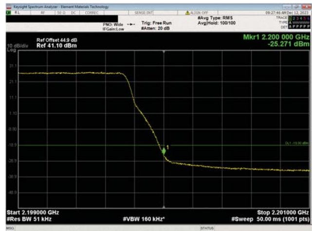
AWS Band n66, 2110 MHz - 2200 MHz 5 MHz Bandwidth 256QAM Modulation High Ch, 2197.5 MHz
