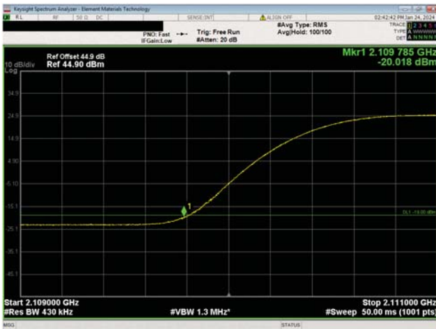
AWS Multicarrier Multiband Test Case 2 QPSK Modulation AWS n66, NR40, Low Ch, 2130.0 MHz
