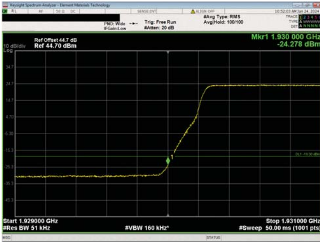
PCS Multicarrier Multiband Test Case 1 QPSK Modulation PCS n25, NR5, Low Ch, 1932.5 MHz
