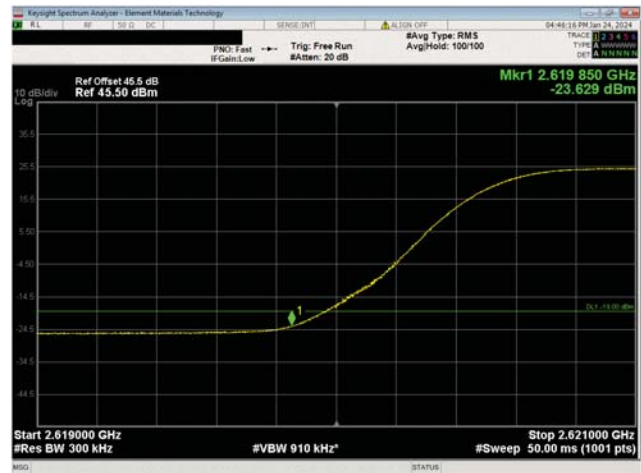
BRS Multicarrier Multiband Test Case 2 QPSK Modulation BRS n7, NR30, Low Ch, 2635.0 MHz
