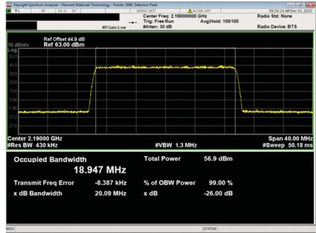
AWS Band n66, 2110 MHz - 2200 MHz 20 MHz Bandwidth 256QAM Modulation High Ch, 2190.0 MHz
