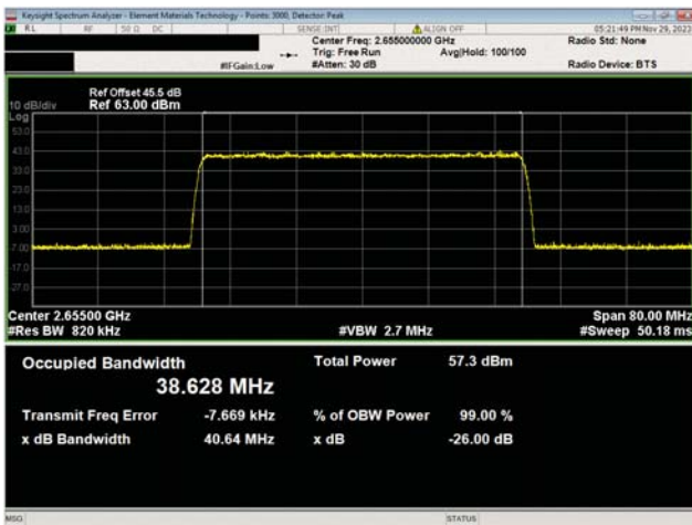
BRS Band n7, 2620 MHz - 2690 MHz 40 MHz Bandwidth 64QAM Modulation Mid Ch, 2655.0 MHz
