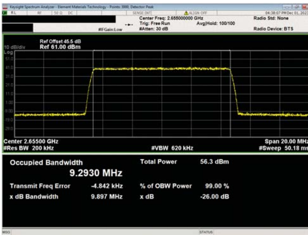
BRS Band n7, 2620 MHz - 2690 MHz 10 MHz Bandwidth QPSK Modulation Mid Ch, 2655.0 MHz
