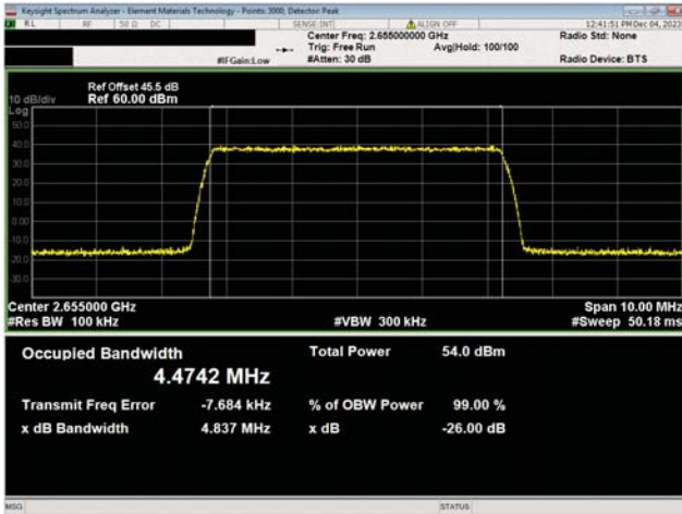
BRS Band n7, 2620 MHz - 2690 MHz 5 MHz Bandwidth QPSK Modulation Mid Ch, 2655.0 MHz
