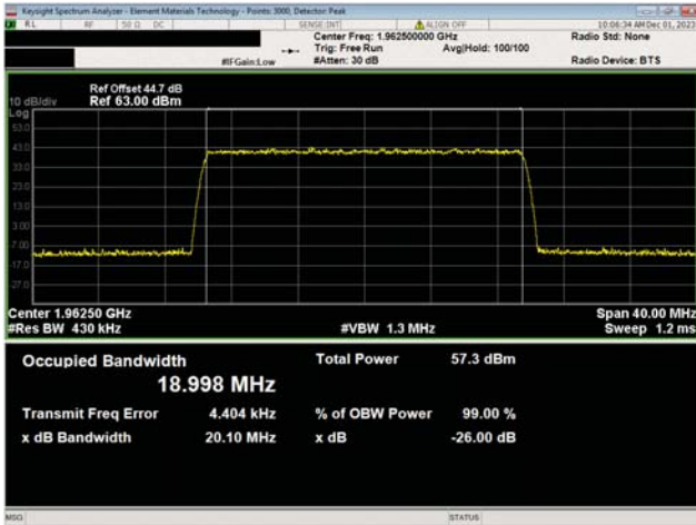
PCS Band n25, 1930 MHz - 1995 MHz 20 MHz Bandwidth 64QAM Modulation Mid Ch, 1962.5 MHz
