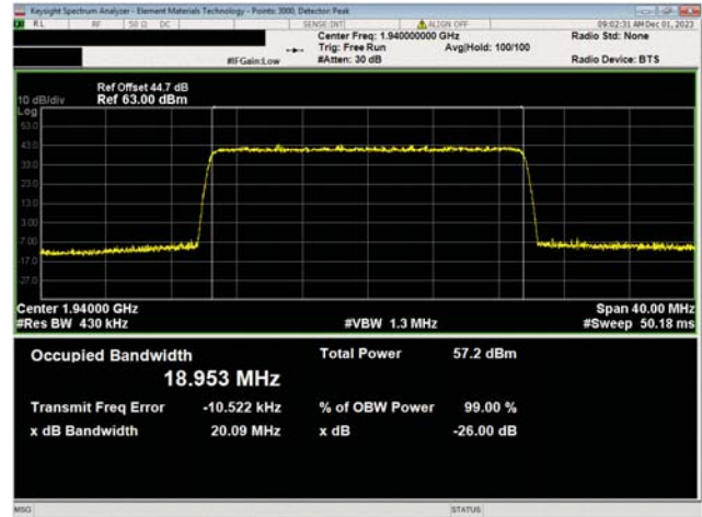
PCS Band n25, 1930 MHz - 1995 MHz 20 MHz Bandwidth 256QAM Modulation Low Ch, 1940.0 MHz
