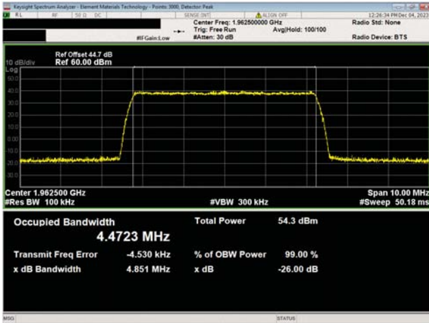
PCS Band n25, 1930 MHz - 1995 MHz 5 MHz Bandwidth QPSK Modulation Mid Ch, 1962.5 MHz
