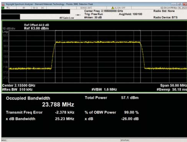
AWS Band n66, 2110 MHz - 2200 MHz 25 MHz Bandwidth 256QAM Modulation Mid Ch, 2155.0 MHz
