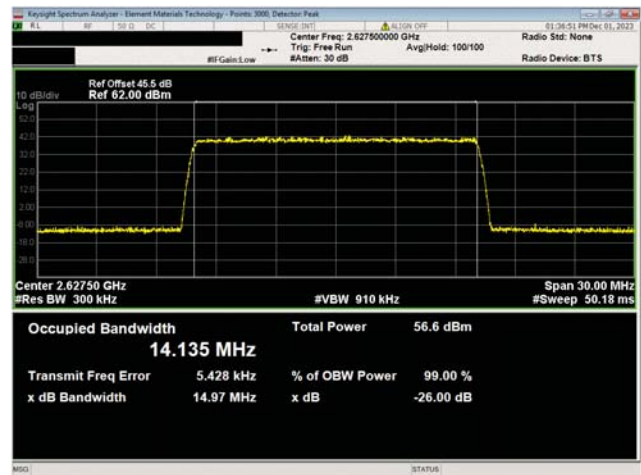
BRS Band n7, 2620 MHz - 2690 MHz 15 MHz Bandwidth 256QAM Modulation Low Ch, 2627.5 MHz
