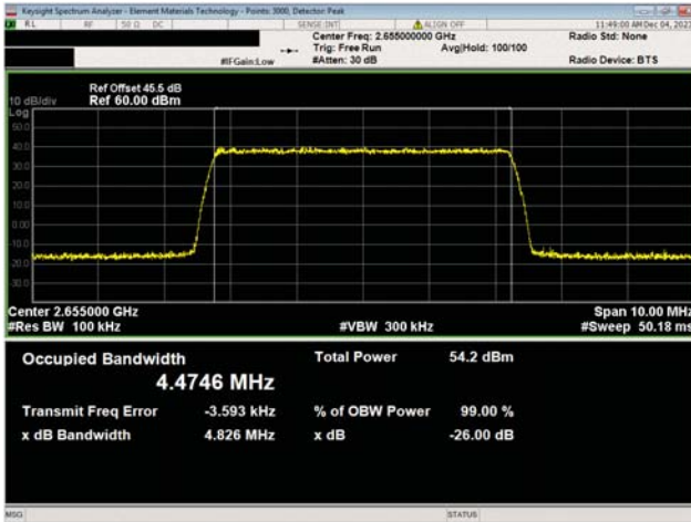
BRS Band n7, 2620 MHz - 2690 MHz 5 MHz Bandwidth 256QAM Modulation Mid Ch, 2655.0 MHz
