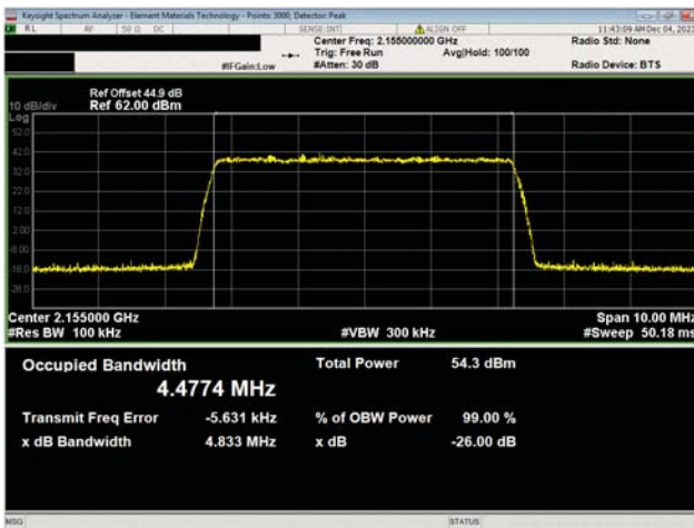
AWS Band n66, 2110 MHz - 2200 MHz 5 MHz Bandwidth 256QAM Modulation Mid Ch, 2155.0 MHz
