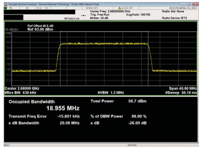
BRS Band n7, 2620 MHz - 2690 MHz 20 MHz Bandwidth 256QAM Modulation High Ch, 2680.0 MHz
