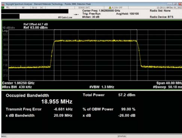
PCS Band n25, 1930 MHz - 1995 MHz 20 MHz Bandwidth QPSK Modulation Mid Ch, 1962.5 MHz
