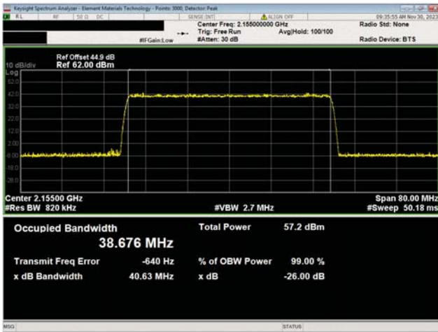
AWS Band n66, 2110 MHz - 2200 MHz 40 MHz Bandwidth QPSK Modulation Mid Ch, 2155.0 MHz
