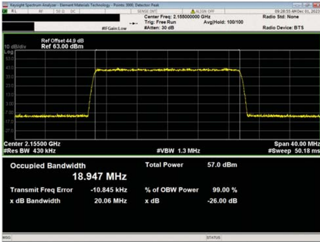
AWS Band n66, 2110 MHz - 2200 MHz 20 MHz Bandwidth 256QAM Modulation Mid Ch, 2155.0 MHz
