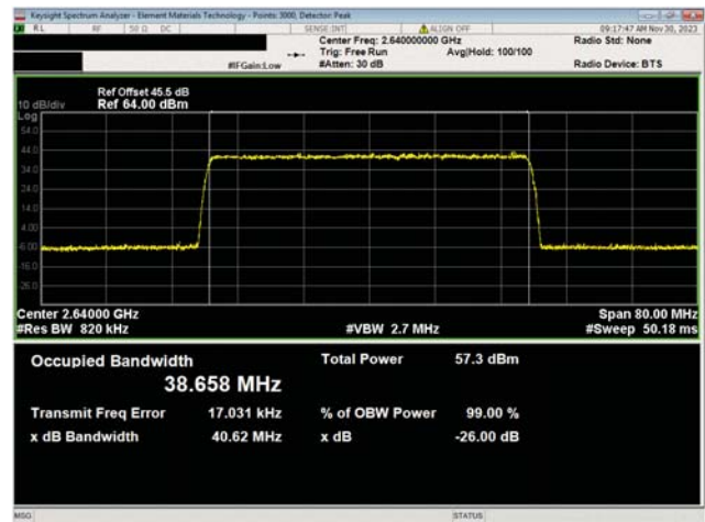
BRS Band n7, 2620 MHz - 2690 MHz 40 MHz Bandwidth 256QAM Modulation Low Ch, 2640.0 MHz
