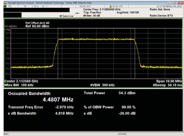
AWS Band n66, 2110 MHz - 2200 MHz 5 MHz Bandwidth 256QAM Modulation Low Ch, 2112.5 MHz
