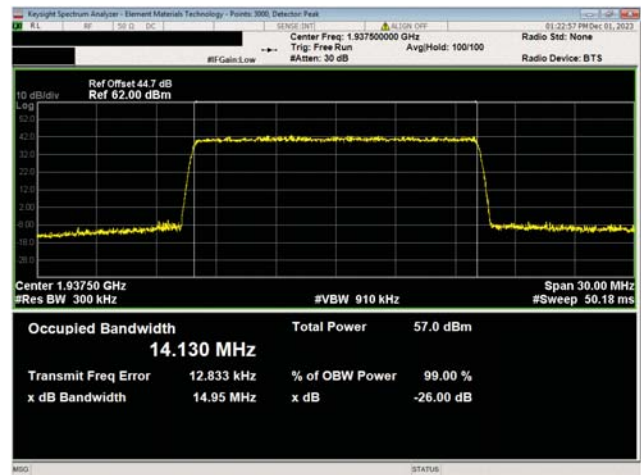
PCS Band n25, 1930 MHz - 1995 MHz 15 MHz Bandwidth 256QAM Modulation Low Ch, 1937.5 MHz
