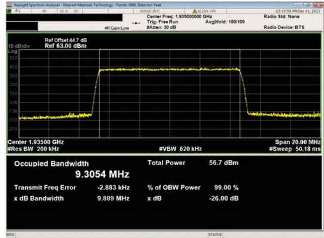
PCS Band n25, 1930 MHz - 1995 MHz 10 MHz Bandwidth 256QAM Modulation Low Ch, 1935.0 MHz
