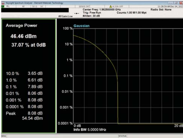
PCS Band n25, 1930 MHz - 1995 MHz 5 MHz Bandwidth 256QAM Modulation Mid Ch, 1962.5 MHz
