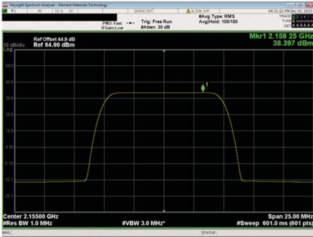
AWS Band n66, 2110 MHz - 2200 MHz 10 MHz Bandwidth QPSK Modulation Mid Ch, 2155.0 MHz
