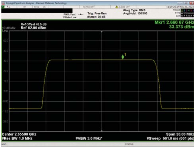
BRS Band n7, 2620 MHz - 2690 MHz 30 MHz Bandwidth QPSK Modulation Mid Ch, 2655.0 MHz
