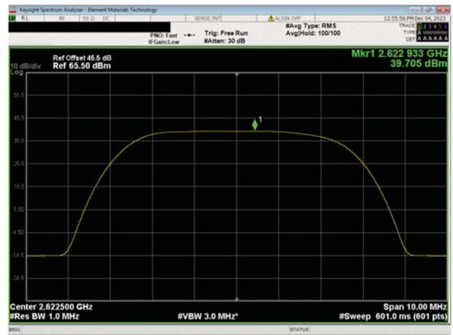
BRS Band n7, 2620 MHz - 2690 MHz 5 MHz Bandwidth 16QAM Modulation Low Ch, 2622.5 MHz
