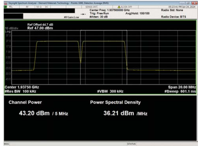
PCS Multicarrier Multiband Test Case 1 QPSK Modulation PSC Band n25, NR5, Low Ch, 1937.5 MHz
