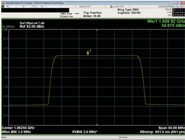
PCS Band n25, 1930 MHz - 1995 MHz 25 MHz Bandwidth QPSK Modulation Mid Ch, 1962.5 MHz
