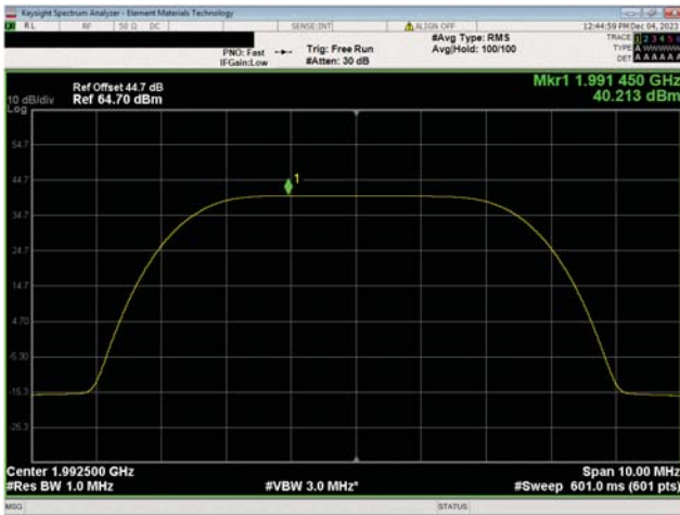
PCS Band n25, 1930 MHz - 1995 MHz 5 MHz Bandwidth QPSK Modulation High Ch, 1992.5 MHz
