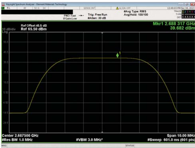
BRS Band n7, 2620 MHz - 2690 MHz 5 MHz Bandwidth QPSK Modulation High Ch, 2687.5 MHz
