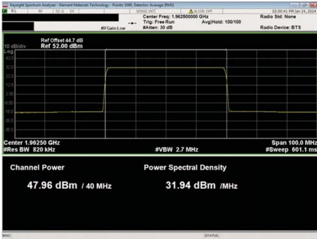
AWS Multicarrier Multiband Test Case 3 QPSK Modulation PSC Band n25, NR40, Mid Ch, 1962.5 MHz
