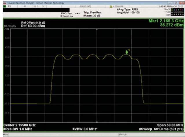
AWS Band n66, 2110 MHz - 2200 MHz 30 MHz Bandwidth 16QAM Modulation Mid Ch, 2155.0 MHz
