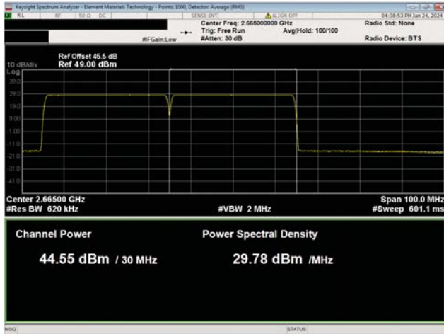
BRS Multicarrier Multiband Test Case 2 QPSK Modulation BRS Band n7, NR30, Low Ch, 2665.0 MHz
