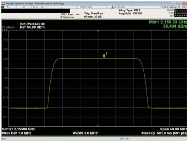
AWS Band n66, 2110 MHz - 2200 MHz 20 MHz Bandwidth 64QAM Modulation Mid Ch, 2155.0 MHz
