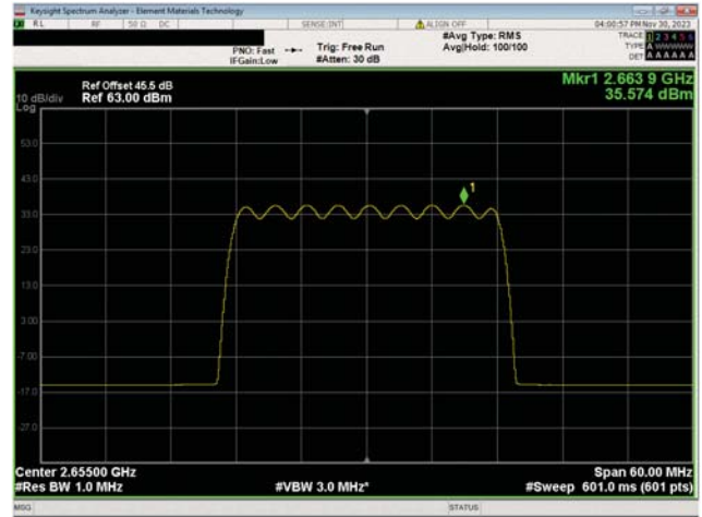
BRS Band n7, 2620 MHz - 2690 MHz 25 MHz Bandwidth 16QAM Modulation Mid Ch, 2655.0 MHz
