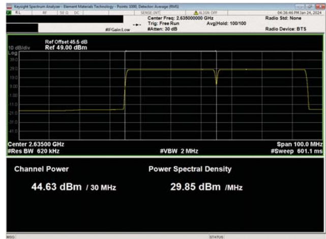
BRS Multicarrier Multiband Test Case 2 QPSK Modulation BRS Band n7, NR30, Low Ch, 2635.0 MHz
