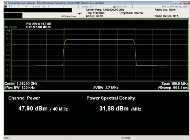
BRS Multicarrier Multiband Test Case 2 QPSK Modulation PSC Band n25, NR40, Mid Ch, 1962.5 MHz
