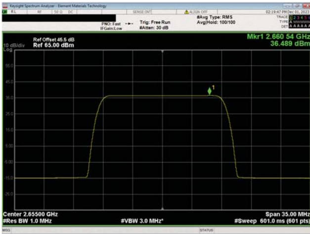
BRS Band n7, 2620 MHz - 2690 MHz 15 MHz Bandwidth 64QAM Modulation Mid Ch, 2655.0 MHz
