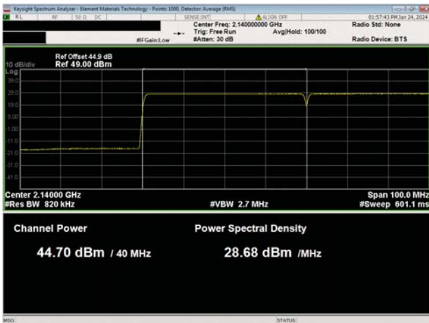
AWS Multicarrier Multiband Test Case 3 QPSK Modulation AWS Band n66, NR40, High Ch, 2140.0 MHz
