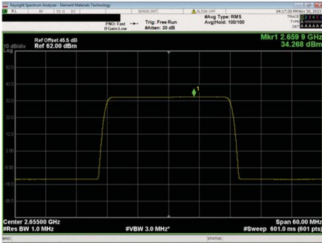
BRS Band n7, 2620 MHz - 2690 MHz 25 MHz Bandwidth QPSK Modulation Mid Ch, 2655.0 MHz
