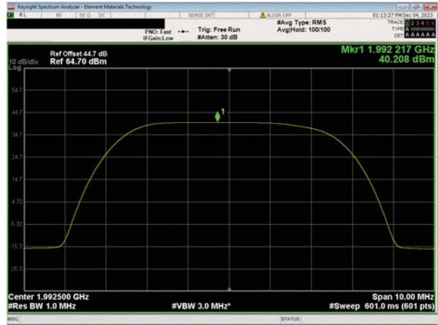
PCS Band n25, 1930 MHz - 1995 MHz 5 MHz Bandwidth 16QAM Modulation High Ch, 1992.5 MHz
