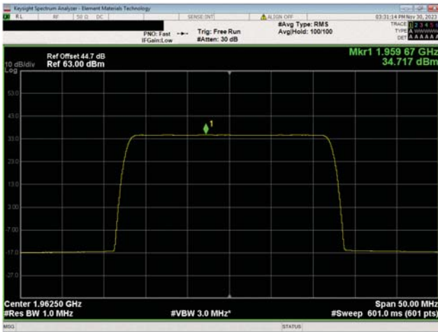
PCS Band n25, 1930 MHz - 1995 MHz 25 MHz Bandwidth 64QAM Modulation Mid Ch, 1962.5 MHz
