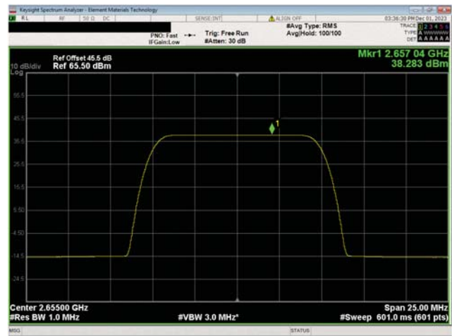
BRS Band n7, 2620 MHz - 2690 MHz 10 MHz Bandwidth 256QAM Modulation Mid Ch, 2655.0 MHz
