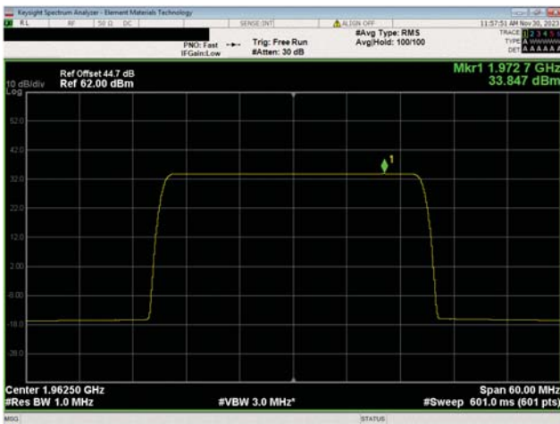
PCS Band n25, 1930 MHz - 1995 MHz 30 MHz Bandwidth 64QAM Modulation Mid Ch, 1962.5 MHz
