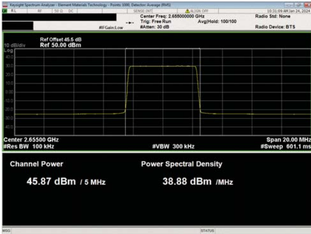
PCS Multicarrier Multiband Test Case 1 QPSK Modulation BRS Band n7, NR5, Mid Ch, 2655.0 MHz
