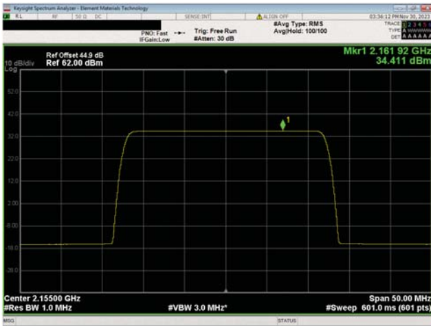
AWS Band n66, 2110 MHz - 2200 MHz 25 MHz Bandwidth 64QAM Modulation Mid Ch, 2155.0 MHz
