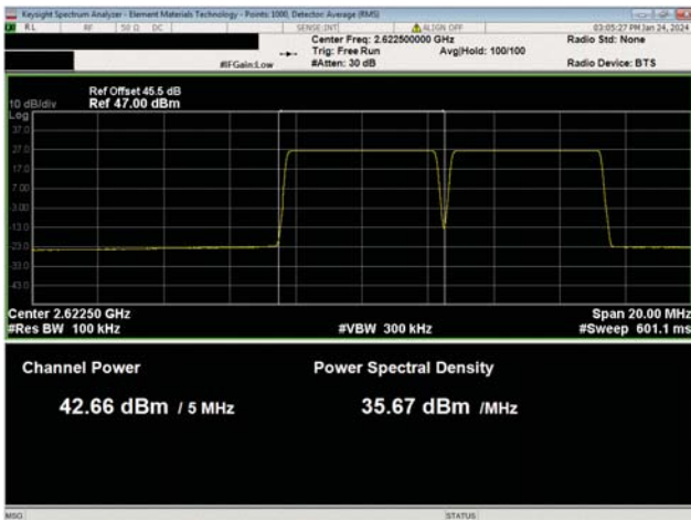
BRS Multicarrier Multiband Test Case 1 QPSK Modulation BRS Band n7, NR5, Low Ch, 2622.5 MHz
