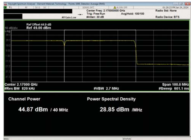
AWS Multicarrier Multiband Test Case 2 QPSK Modulation AWS Band n66, NR40, Low Ch, 2170.0 MHz
