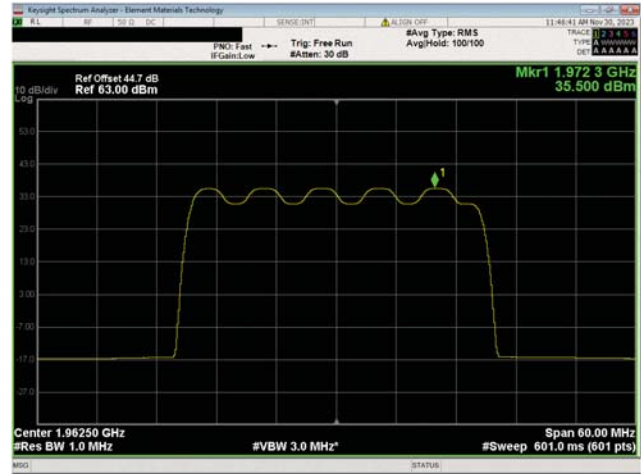
PCS Band n25, 1930 MHz - 1995 MHz 30 MHz Bandwidth 16QAM Modulation Mid Ch, 1962.5 MHz
