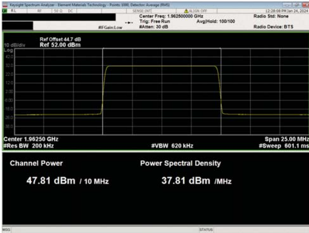
AWS Multicarrier Multiband Test Case 1 QPSK Modulation PSC Band n25, NR10, Mid Ch, 1962.5 MHz
