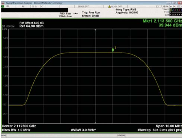
AWS Band n66, 2110 MHz - 2200 MHz 5 MHz Bandwidth QPSK Modulation Low Ch, 2112.5 MHz
