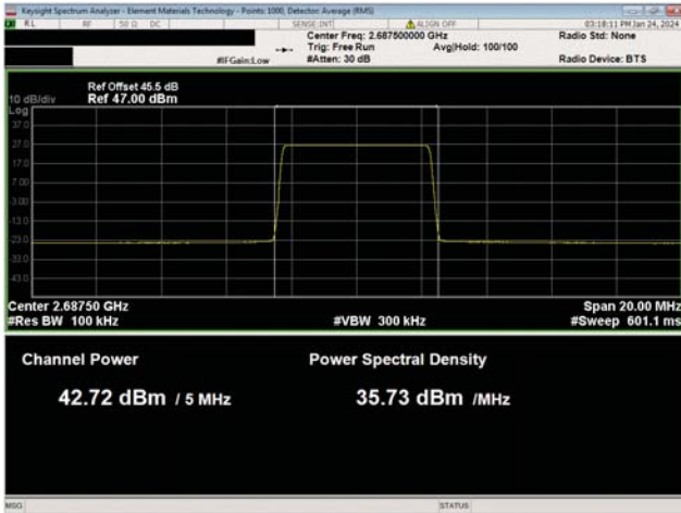
BRS Multicarrier Multiband Test Case 1 QPSK Modulation BRS Band n7, NR5, High Ch, 2687.5 MHz
