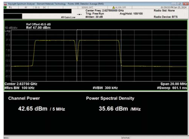
BRS Multicarrier Multiband Test Case 1 QPSK Modulation BRS Band n7, NR5, Low Ch, 2627.5 MHz
