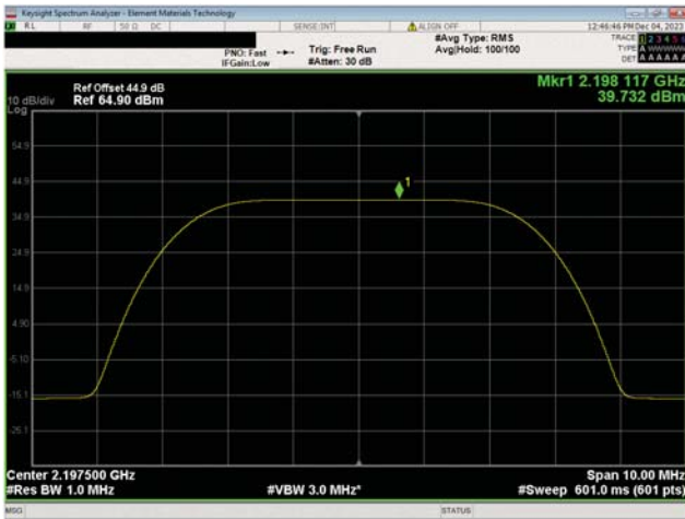
AWS Band n66, 2110 MHz - 2200 MHz 5 MHz Bandwidth QPSK Modulation High Ch, 2197.5 MHz
