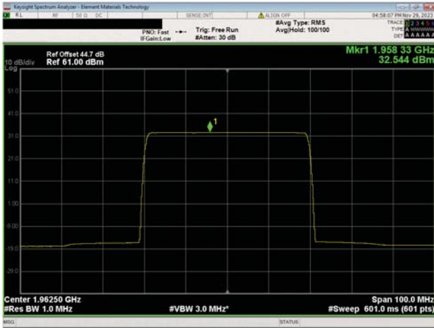
PCS Band n25, 1930 MHz - 1995 MHz 40 MHz Bandwidth QPSK Modulation Mid Ch, 1962.5 MHz
