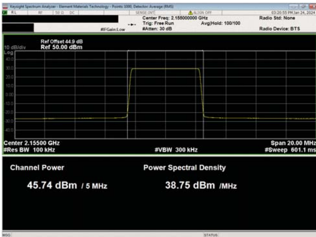
BRS Multicarrier Multiband Test Case 1 QPSK Modulation AWS Band n66, NR5, Mid Ch, 2155.0 MHz
