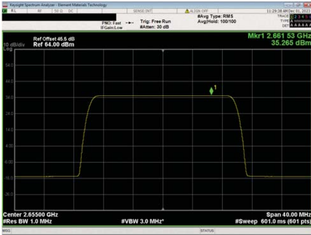
BRS Band n7, 2620 MHz - 2690 MHz 20 MHz Bandwidth QPSK Modulation Mid Ch, 2655.0 MHz
