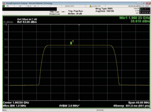
PCS Band n25, 1930 MHz - 1995 MHz 20 MHz Bandwidth 256QAM Modulation Mid Ch, 1962.5 MHz
