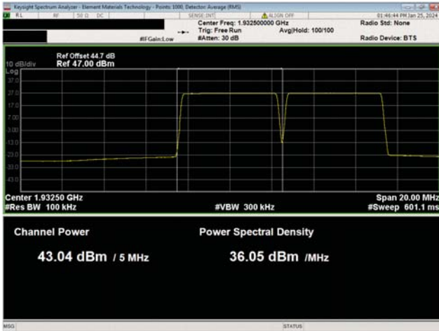
PCS Multicarrier Multiband Test Case 1 QPSK Modulation PSC Band n25, NR5, Low Ch, 1932.5 MHz
