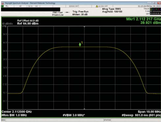
AWS Band n66, 2110 MHz - 2200 MHz 5 MHz Bandwidth 64QAM Modulation Low Ch, 2112.5 MHz
