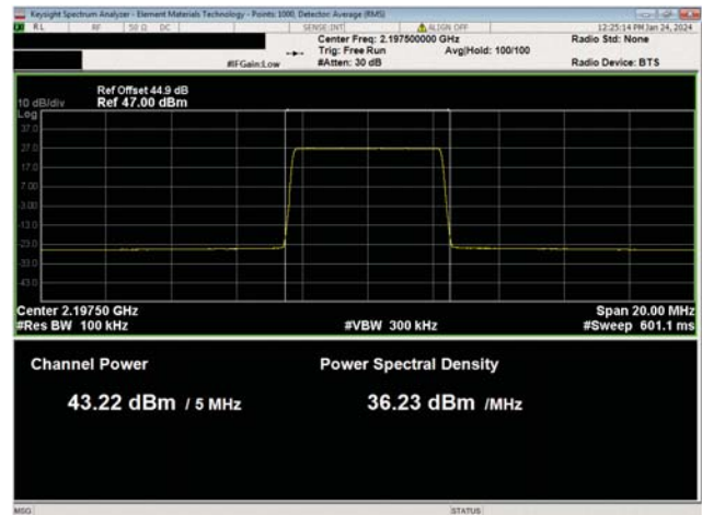
AWS Multicarrier Multiband Test Case 1 QPSK Modulation AWS Band n66, NR5, High Ch, 2197.5 MHz
