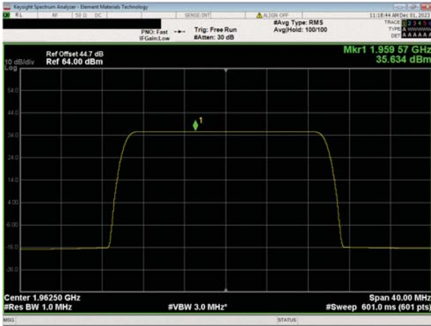
PCS Band n25, 1930 MHz - 1995 MHz 20 MHz Bandwidth QPSK Modulation Mid Ch, 1962.5 MHz
