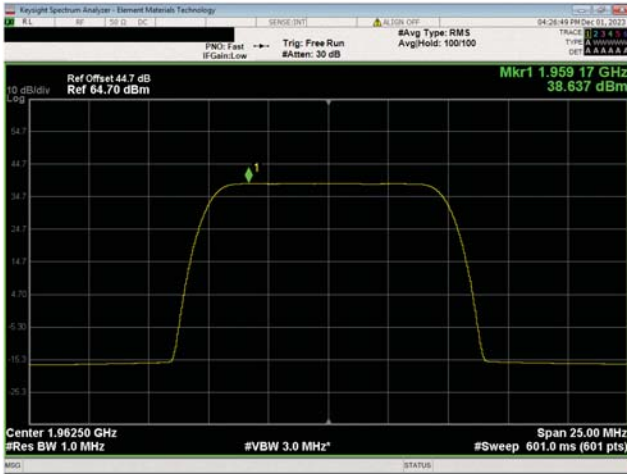
PCS Band n25, 1930 MHz - 1995 MHz 10 MHz Bandwidth QPSK Modulation Mid Ch, 1962.5 MHz
