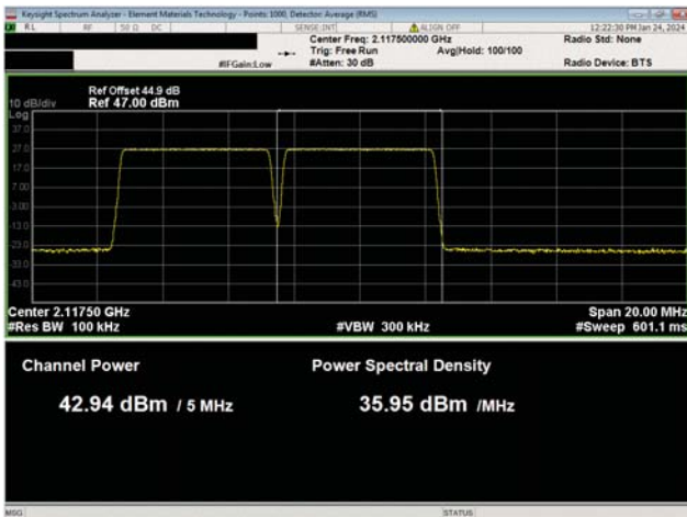
AWS Multicarrier Multiband Test Case 1 QPSK Modulation AWS Band n66, NR5, Low Ch, 2117.5 MHz
