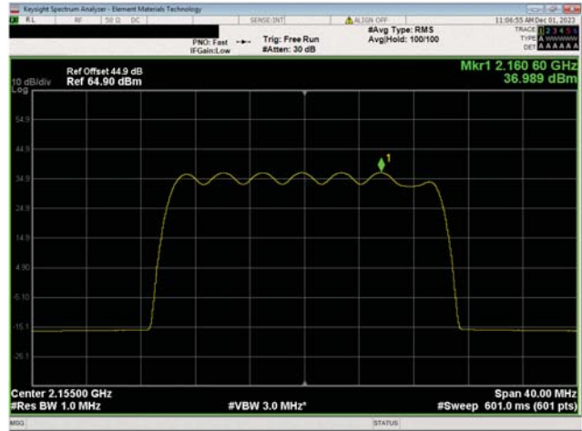
AWS Band n66, 2110 MHz - 2200 MHz 20 MHz Bandwidth 16QAM Modulation Mid Ch, 2155.0 MHz
