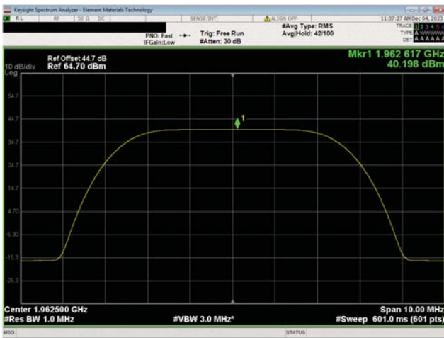
PCS Band n25, 1930 MHz - 1995 MHz 5 MHz Bandwidth 256QAM Modulation Mid Ch, 1962.5 MHz
