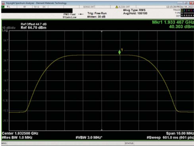
PCS Band n25, 1930 MHz - 1995 MHz 5 MHz Bandwidth QPSK Modulation Low Ch, 1932.5 MHz
