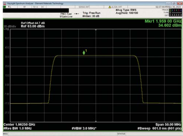
PCS Band n25, 1930 MHz - 1995 MHz 25 MHz Bandwidth 256QAM Modulation Mid Ch, 1962.5 MHz
