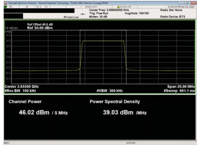
AWS Multicarrier Multiband Test Case 1 QPSK Modulation BRS Band n7, NR5, Mid Ch, 2655.0 MHz
