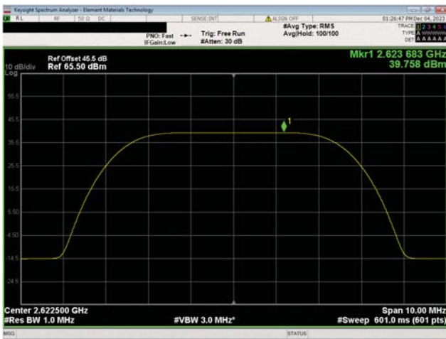
BRS Band n7, 2620 MHz - 2690 MHz 5 MHz Bandwidth 64QAM Modulation Low Ch, 2625.0 MHz
