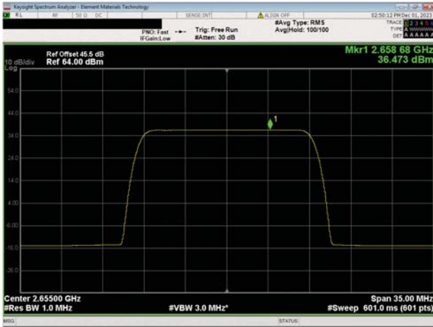
BRS Band n7, 2620 MHz - 2690 MHz 15 MHz Bandwidth QPSK Modulation Mid Ch, 2655.0 MHz
