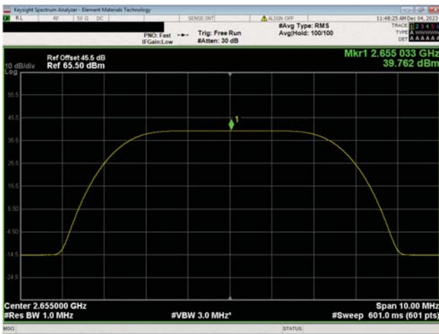
BRS Band n7, 2620 MHz - 2690 MHz 5 MHz Bandwidth 256QAM Modulation Mid Ch, 2655.0 MHz
