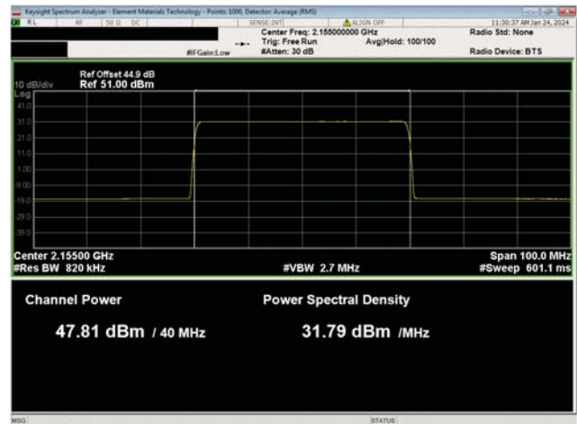
PCS Multicarrier Multiband Test Case 2 QPSK Modulation AWS Band n66, NR40, Mid Ch, 2155.0 MHz
