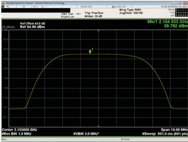
AWS Band n66, 2110 MHz - 2200 MHz 5 MHz Bandwidth 16QAM Modulation Mid Ch, 2155.0 MHz
