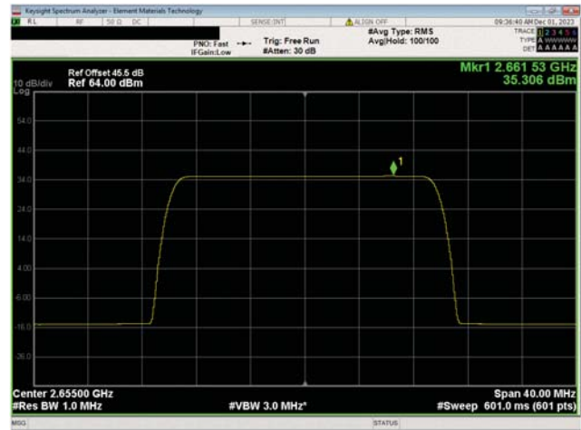
BRS Band n7, 2620 MHz - 2690 MHz 20 MHz Bandwidth 256QAM Modulation Mid Ch, 2655.0 MHz
