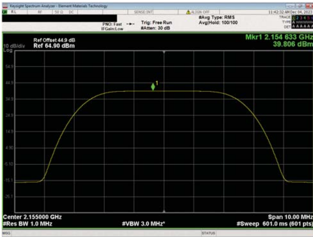
AWS Band n66, 2110 MHz - 2200 MHz 5 MHz Bandwidth 256QAM Modulation Mid Ch, 2155.0 MHz
