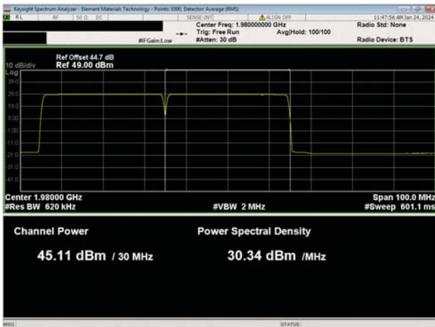
PCS Multicarrier Multiband Test Case 3 QPSK Modulation PSC Band n25, NR30, High Ch, 1980.0 MHz
