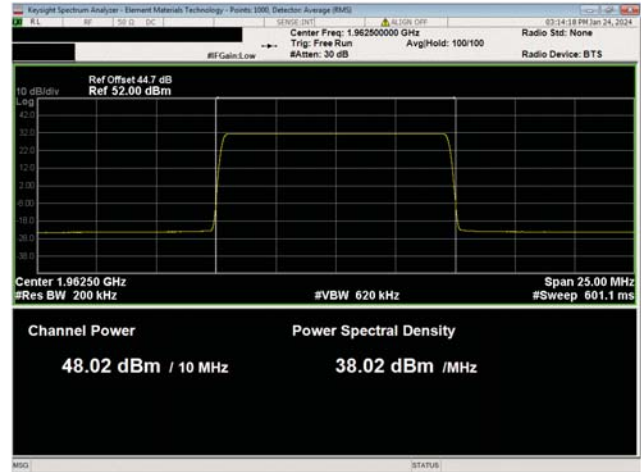
BRS Multicarrier Multiband Test Case 1 QPSK Modulation PSC Band n25, NR10, Mid Ch, 1962.5 MHz
