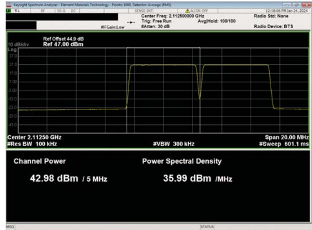
AWS Multicarrier Multiband Test Case 1 QPSK Modulation AWS Band n66, NR5, Low Ch, 2112.5 MHz
