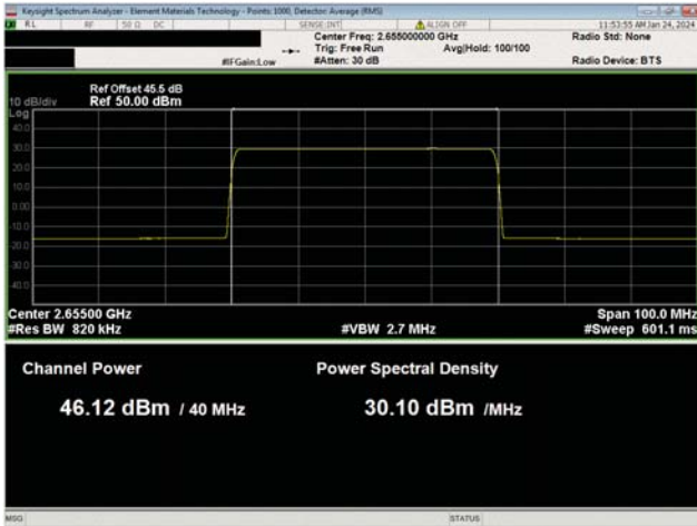
PCS Multicarrier Multiband Test Case 3 QPSK Modulation BRS Band n7, NR40, Mid Ch, 2655.0 MHz
