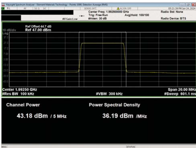
PCS Multicarrier Multiband Test Case 1 QPSK Modulation PSC Band n25, NR5, High Ch, 1992.5 MHz
