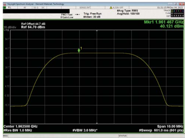
PCS Band n25, 1930 MHz - 1995 MHz 5 MHz Bandwidth 64QAM Modulation Mid Ch, 1962.5 MHz
