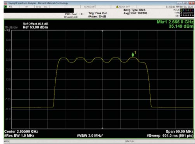
BRS Band n7, 2620 MHz - 2690 MHz 30 MHz Bandwidth 16QAM Modulation Mid Ch, 2655.0 MHz
