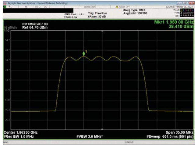
PCS Band n25, 1930 MHz - 1995 MHz 15 MHz Bandwidth 16QAM Modulation Mid Ch, 1962.5 MHz
