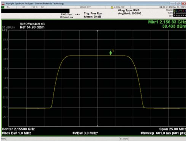
AWS Band n66, 2110 MHz - 2200 MHz 10 MHz Bandwidth 64QAM Modulation Mid Ch, 2155.0 MHz
