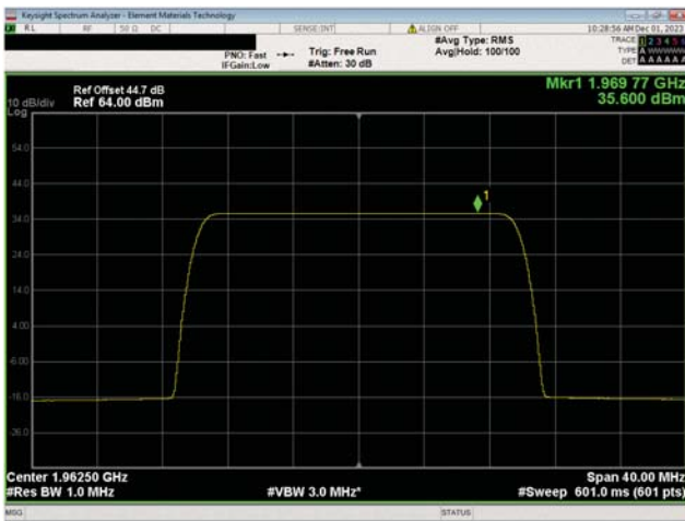
PCS Band n25, 1930 MHz - 1995 MHz 20 MHz Bandwidth 64QAM Modulation Mid Ch, 1962.5 MHz
