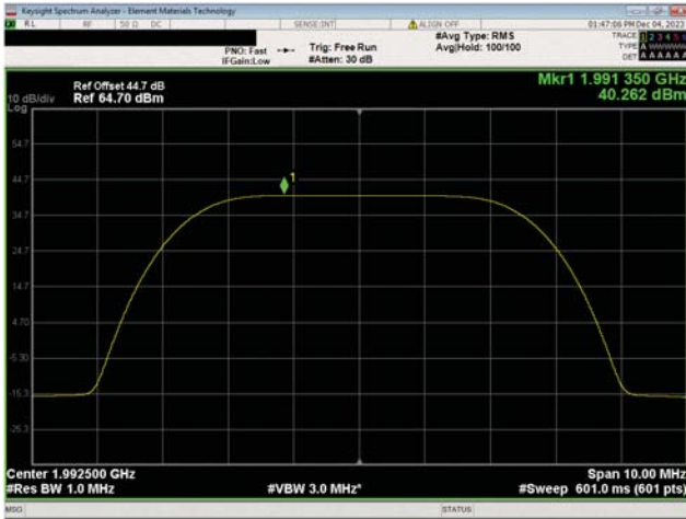
PCS Band n25, 1930 MHz - 1995 MHz 5 MHz Bandwidth 64QAM Modulation High Ch, 1992.5 MHz
