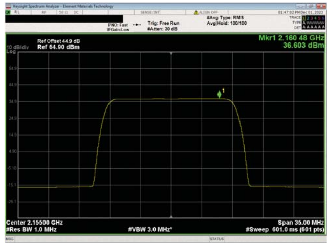
AWS Band n66, 2110 MHz - 2200 MHz 15 MHz Bandwidth 256QAM Modulation Mid Ch, 2155.0 MHz
