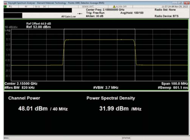
AWS Band n66, 2110-2200 MHz 40 MHz Bandwidth 256QAM Modulation Mid Channel, 2155.0 MHz Port 2
