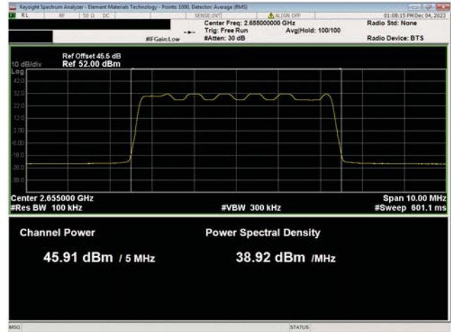
BRS Band n7, 2620 Mhz - 2690 MHz 5 MHz Bandwidth 16QAM Modulation Mid Ch, 2655.0 MHz
