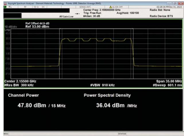
AWS Band n66, 2110 Mhz - 2200 MHz 15 MHz Bandwidth 16QAM Modulation Mid Ch, 2155.0 MHz
