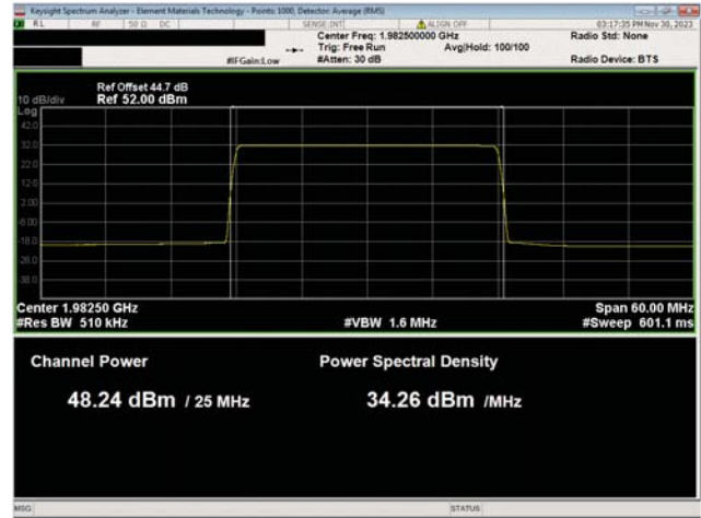
PCS Band n25, 1930 MHz - 1995 MHz 25 MHz Bandwidth 256QAM Modulation High Ch, 1982.5 MHz
