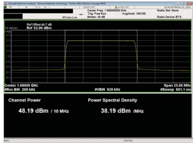
PCS Band n25, 1930 MHz - 1995 MHz 10 MHz Bandwidth 256QAM Modulation High Ch, 1990.0 MHz
