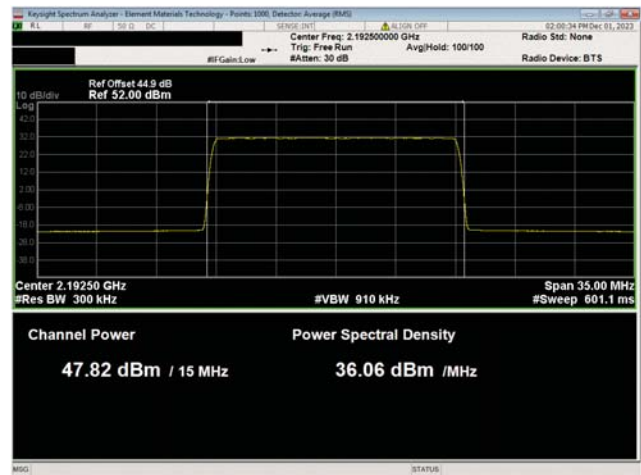
AWS Band n66, 2110 Mhz - 2200 MHz 15 MHz Bandwidth 15 MHz Bandwidth 256QAM Modulation High Ch, 2192.5 MHz
