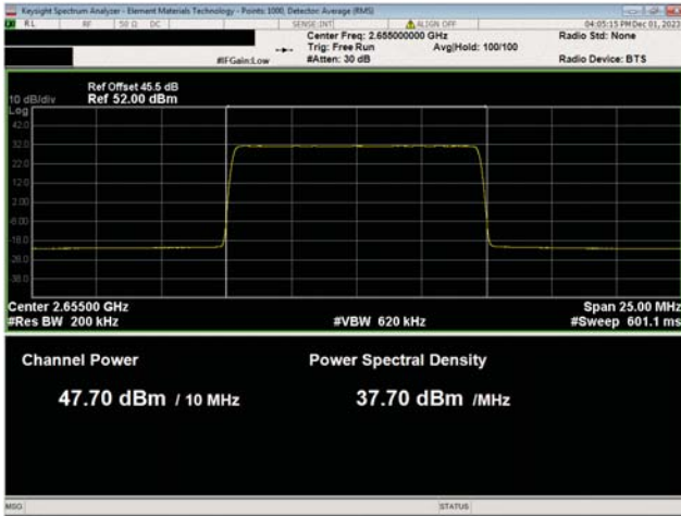
BRS Band n7, 2620 Mhz - 2690 MHz 10 MHz Bandwidth 64QAM Modulation Mid Ch, 2655.0 MHz
