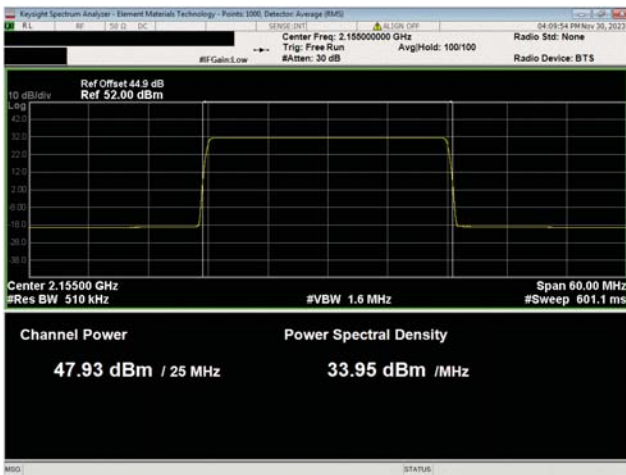
AWS Band n66, 2110 Mhz - 2200 MHz 25 MHz Bandwidth QPSK Modulation Mid Ch, 2155.0 MHz
