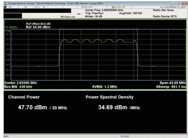
BRS Band n7, 2620 Mhz - 2690 MHz 20 MHz Bandwidth 16QAM Modulation Mid Ch, 2655.0 MHz
