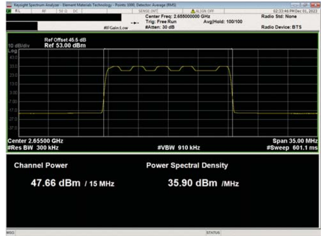
BRS Band n7, 2620 Mhz - 2690 MHz 15 MHz Bandwidth 16QAM Modulation Mid Ch, 2655.0 MHz
