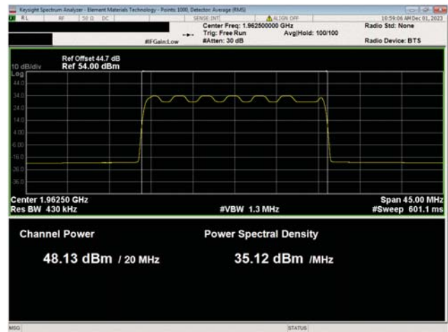
PCS Band n25, 1930 MHz - 1995 MHz 20 MHz Bandwidth 16QAM Modulation Mid Ch, 1962.5 MHz
