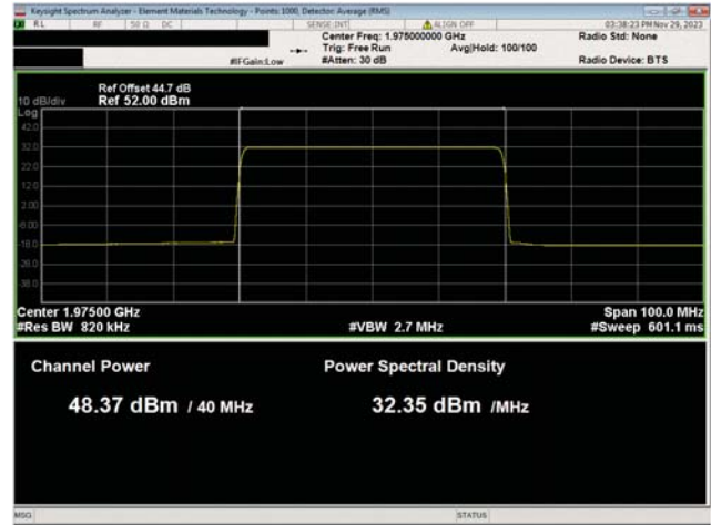
PCS Band n25, 1930 MHz - 1995 MHz 40 MHz Bandwidth 256QAM Modulation High Ch, 1975.0 MHz
