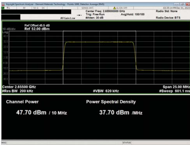
BRS Band n7, 2620 Mhz - 2690 MHz 10 MHz Bandwidth 256QAM Modulation Mid Ch, 2655.0 MHz
