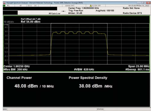
PCS Band n25, 1930 MHz - 1995 MHz 10 MHz Bandwidth 16QAM Modulation Mid Ch, 1962.5 MHz
