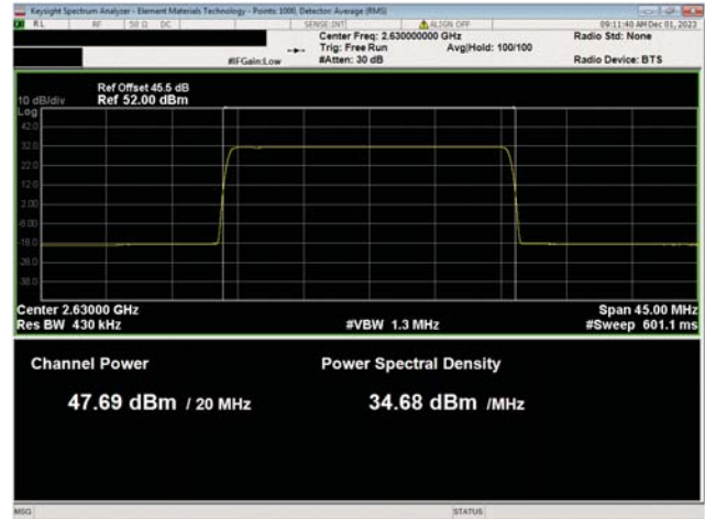
BRS Band n7, 2620 Mhz - 2690 MHz 20 MHz Bandwidth 256QAM Modulation Low Ch, 2630.0 MHz
