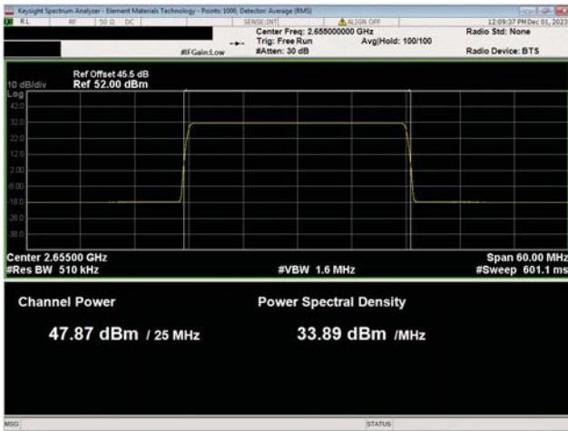
BRS Band n7, 2620 Mhz - 2690 MHz 25 MHz Bandwidth 64QAM Modulation Mid Ch, 2655.0 MHz
