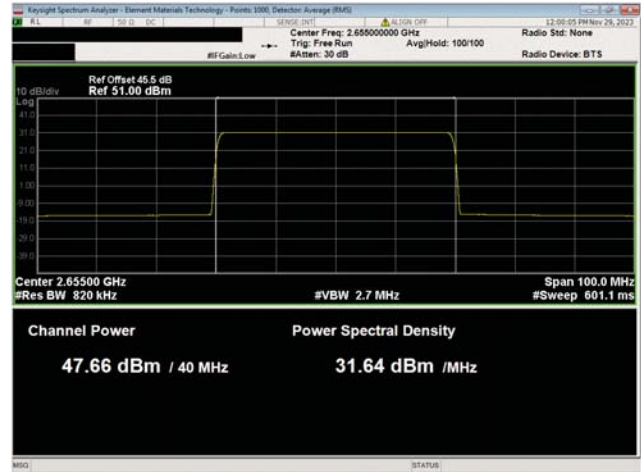
BRS Band n7, 2620-2690 MHz 40 MHz Bandwidth 256QAM Modulation Mid Channel, 2655.0 MHz Port 2
