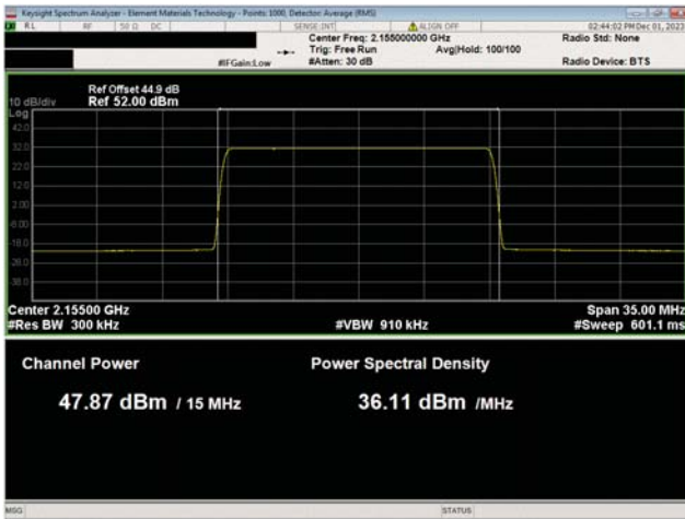
AWS Band n66, 2110 Mhz - 2200 MHz 15 MHz Bandwidth QPSK Modulation Mid Ch, 2155.0 MHz
