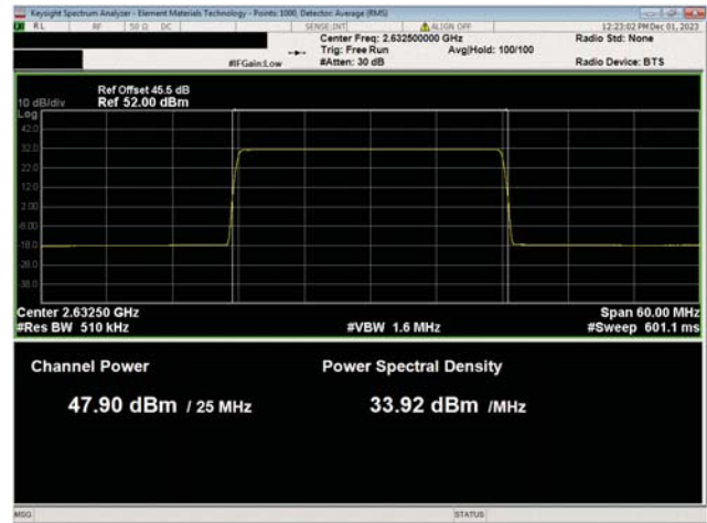
BRS Band n7, 2620 Mhz - 2690 MHz 25 MHz Bandwidth 256QAM Modulation Low Ch, 2632.5 MHz
