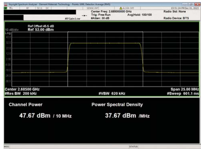
BRS Band n7, 2620 Mhz - 2690 MHz 10 MHz Bandwidth 256QAM Modulation High Ch, 2685.0 MHz
