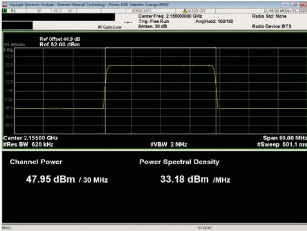
AWS Band n66, 2110 Mhz - 2200 MHz 30 MHz Bandwidth 256QAM Modulation Mid Ch, 2155.0 MHz
