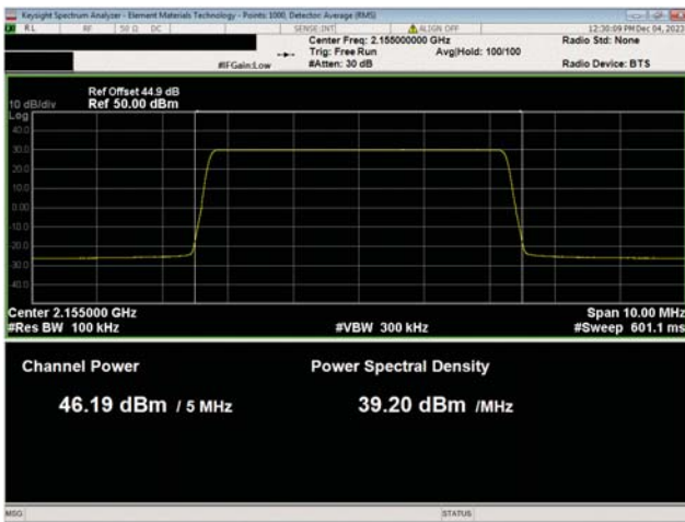
AWS Band n66, 2110 Mhz - 2200 MHz 5 MHz Bandwidth QPSK Modulation Mid Ch, 2155.0 MHz
