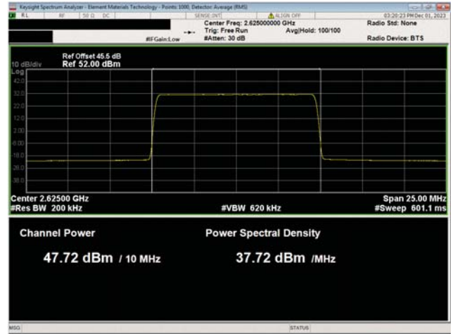
BRS Band n7, 2620 Mhz - 2690 MHz 10 MHz Bandwidth 256QAM Modulation Low Ch, 2625.0 MHz
