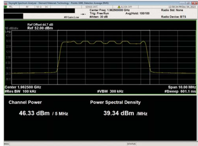
PCS Band n25, 1930 MHz - 1995 MHz 5 MHz Bandwidth 16QAM Modulation Mid Ch, 1962.5 MHz
