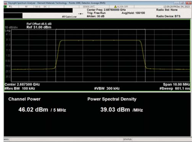
BRS Band n7, 2620 MHz - 2690 MHz 5 MHz Bandwidth 256QAM Modulation High Ch, 2687.5 MHz
