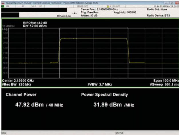
AWS Band n66, 2110-2200 MHz 40 MHz Bandwidth 256QAM Modulation Mid Channel, 2155.0 MHz Port 1
