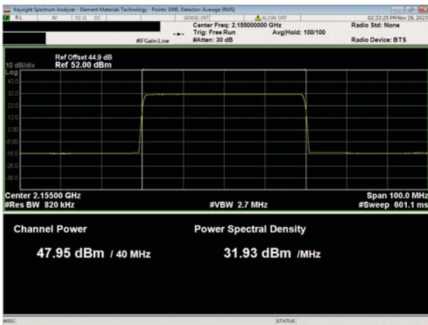
AWS Band n66, 2110 Mhz - 2200 MHz 40 MHz Bandwidth 256QAM Modulation Mid Ch, 2155.0 MHz
