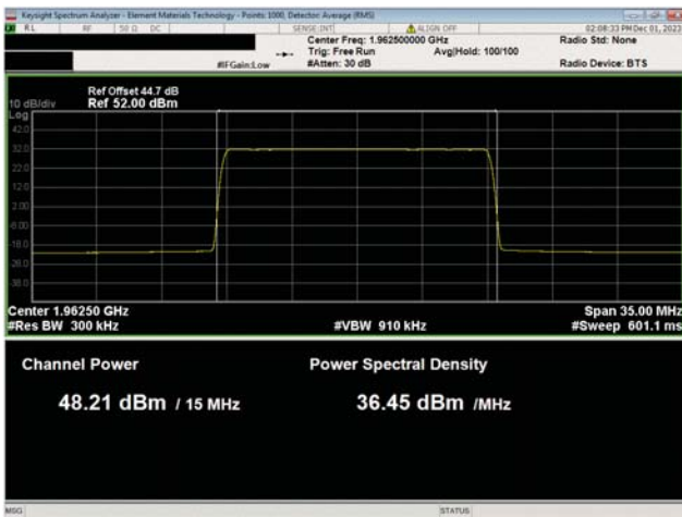
PCS Band n25, 1930 MHz - 1995 MHz 15 MHz Bandwidth 64QAM Modulation Mid Ch, 1962.5 MHz
