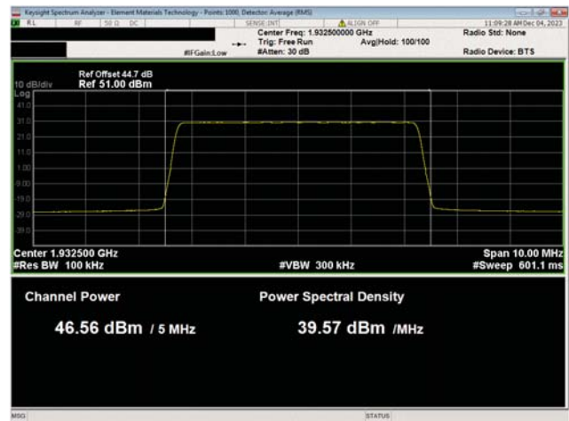
PCS Band n25, 1930 MHz - 1995 MHz 5 MHz Bandwidth 256QAM Modulation Low Ch, 1932.5 MHz
