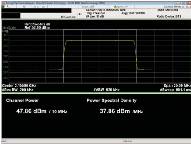
AWS Band n66, 2110 Mhz - 2200 MHz 10 MHz Bandwidth 256QAM Modulation Mid Ch, 2155.0 MHz
