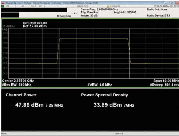
BRS Band n7, 2620 Mhz - 2690 MHz 25 MHz Bandwidth 256QAM Modulation Mid Ch, 2655.0 MHz
