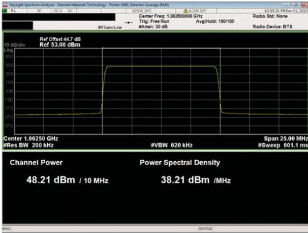
PCS Band n25, 1930 MHz - 1995 MHz 10 MHz Bandwidth 64QAM Modulation Mid Ch, 1962.5 MHz
