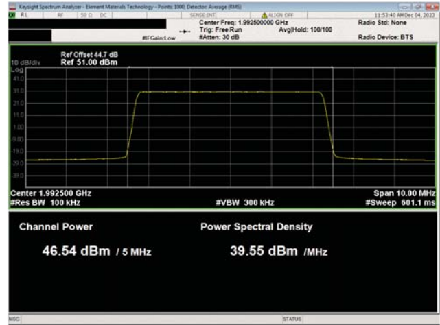
PCS Band n25, 1930 MHz - 1995 MHz 5 MHz Bandwidth 256QAM Modulation High Ch, 1992.5 MHz
