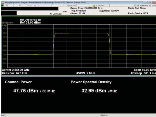
BRS Band n7, 2620 Mhz - 2690 MHz 30 MHz Bandwidth 64QAM Modulation Mid Ch, 2655.0 MHz
