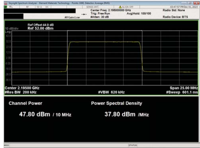
AWS Band n66, 2110 Mhz - 2200 MHz 10 MHz Bandwidth 256QAM Modulation High Ch, 2195.0 MHz
