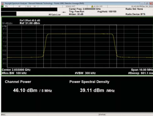
BRS Band n7, 2620 Mhz - 2690 MHz 5 MHz Bandwidth 64QAM Modulation Mid Ch, 2655.0 MHz
