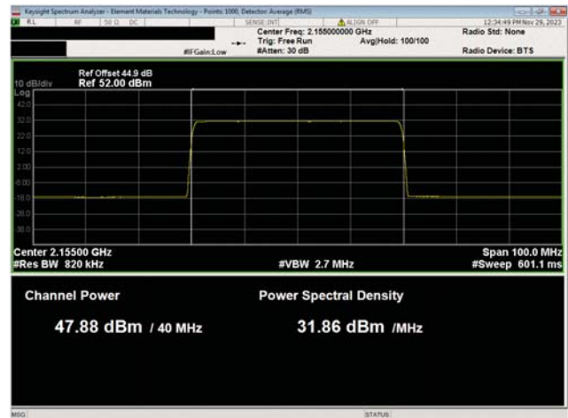
AWS Band n66, 2110-2200 MHz 40 MHz Bandwidth 256QAM Modulation Mid Channel, 2155.0 MHz Port 4
