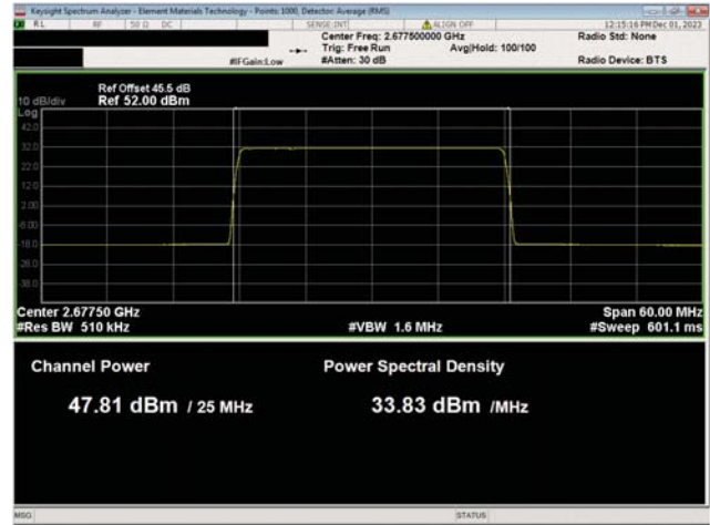
BRS Band n7, 2620 Mhz - 2690 MHz 25 MHz Bandwidth 256QAM Modulation High Ch, 2677.5 MHz
