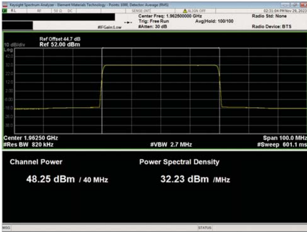
PCS Band n25, 1930 MHz - 1995 MHz 40 MHz Bandwidth 256QAM Modulation Mid Ch, 1962.5 MHz
