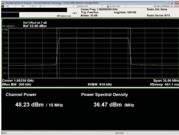
PCS Band n25, 1930 MHz - 1995 MHz 15 MHz Bandwidth QPSK Modulation Mid Ch, 1962.5 MHz
