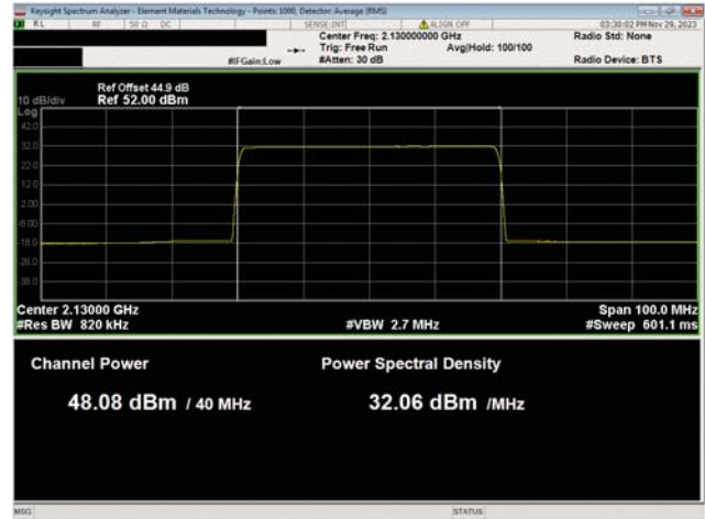
AWS Band n66, 2110 Mhz - 2200 MHz 40 MHz Bandwidth 256QAM Modulation Low Ch, 2130.0 MHz
