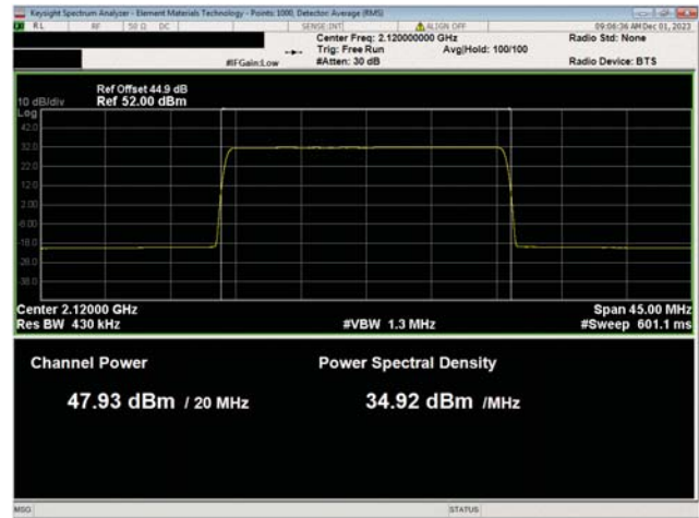
AWS Band n66, 2110 Mhz - 2200 MHz 20 MHz Bandwidth 256QAM Modulation Low Ch, 2120.0 MHz
