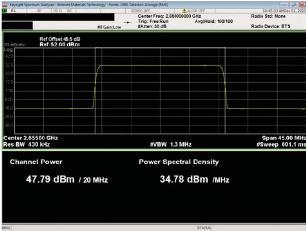
BRS Band n7, 2620 Mhz - 2690 MHz 20 MHz Bandwidth 64QAM Modulation Mid Ch, 2655.0 MHz
