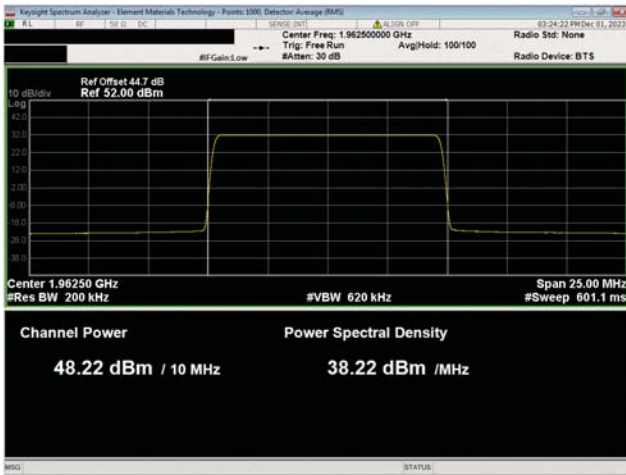
PCS Band n25, 1930 MHz - 1995 MHz 10 MHz Bandwidth 256QAM Modulation Mid Ch, 1962.5 MHz
