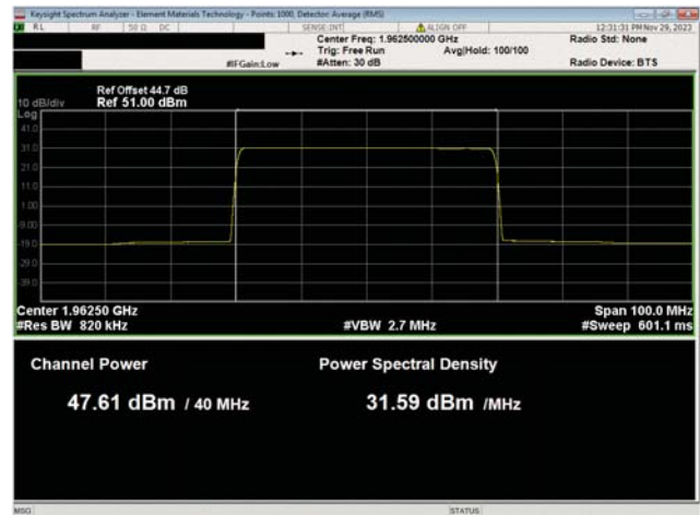
PCS Band n25, 1930-1995 MHz 40 MHz Bandwidth 256QAM Modulation Mid Channel, 1962.5 MHz Port 4
