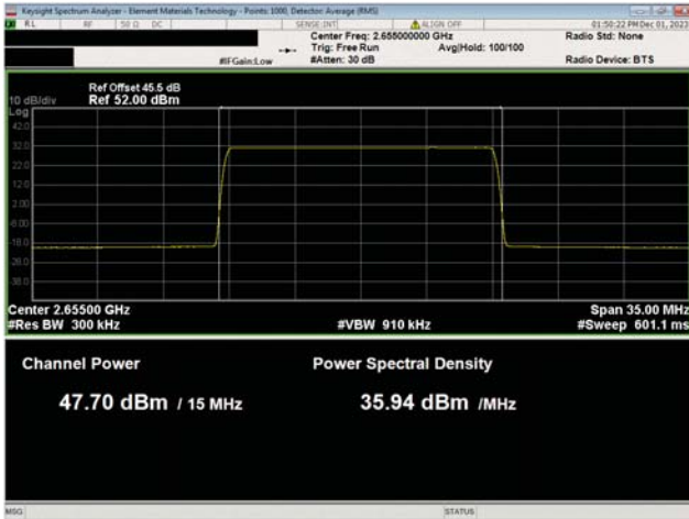
BRS Band n7, 2620 Mhz - 2690 MHz 15 MHz Bandwidth 256QAM Modulation Mid Ch, 2655.0 MHz
