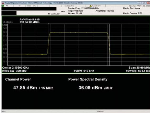
AWS Band n66, 2110 Mhz - 2200 MHz 15 MHz Bandwidth 64QAM Modulation Mid Ch, 2155.0 MHz
