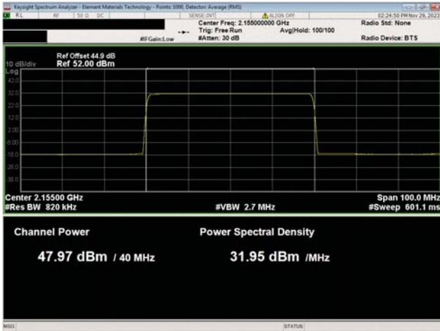
AWS Band n66, 2110 Mhz - 2200 MHz 40 MHz Bandwidth 64QAM Modulation Mid Ch, 2155.0 MHz
