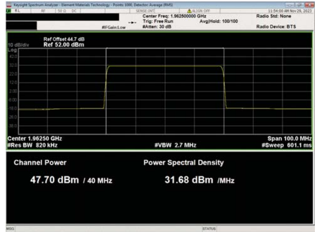
PCS Band n25, 1930-1995 MHz 40 MHz Bandwidth 256QAM Modulation Mid Channel, 1962.5 MHz Port 2
