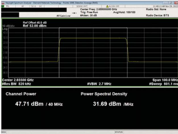
BRS Band n7, 2620-2690 MHz 40 MHz Bandwidth 256QAM Modulation Mid Channel, 2655.0 MHz Port 1
