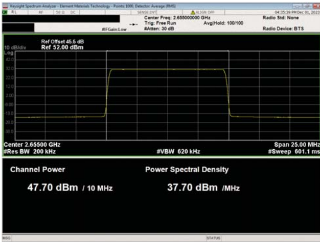
BRS Band n7, 2620 MHz - 2690 MHz 10 MHz Bandwidth QPSK Modulation Mid Ch, 2655.0 MHz
