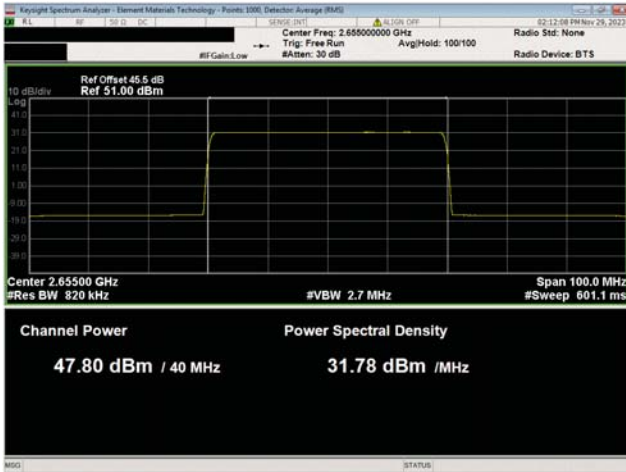
BRS Band n7, 2620 Mhz - 2690 MHz 40 MHz Bandwidth QPSK Modulation Mid Ch, 2655.0 MHz
