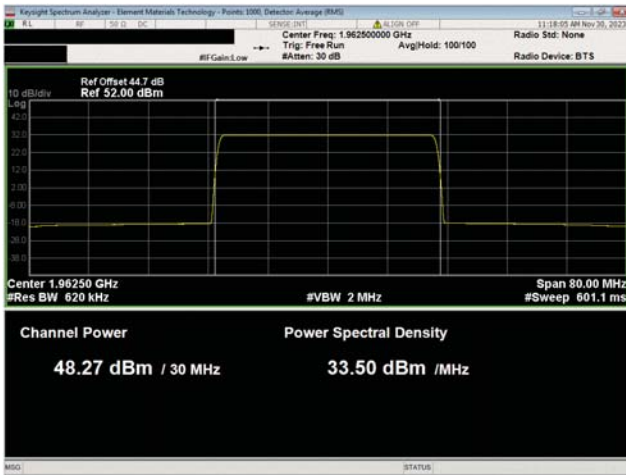
PCS Band n25, 1930 MHz - 1995 MHz 30 MHz Bandwidth QPSK Modulation Mid Ch, 1962.5 MHz
