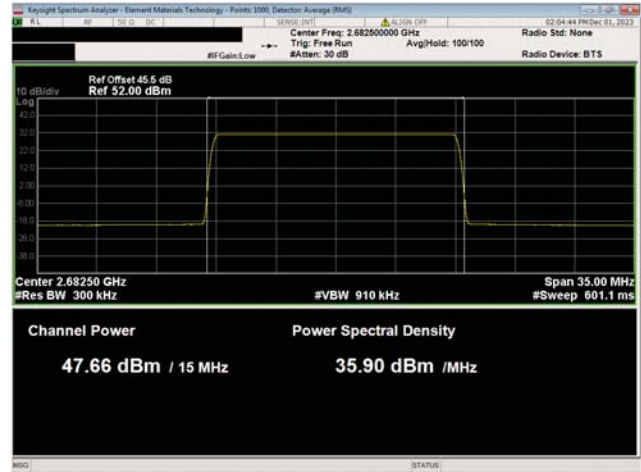
BRS Band n7, 2620 Mhz - 2690 MHz 15 MHz Bandwidth 256QAM Modulation High Ch, 2682.5 MHz
