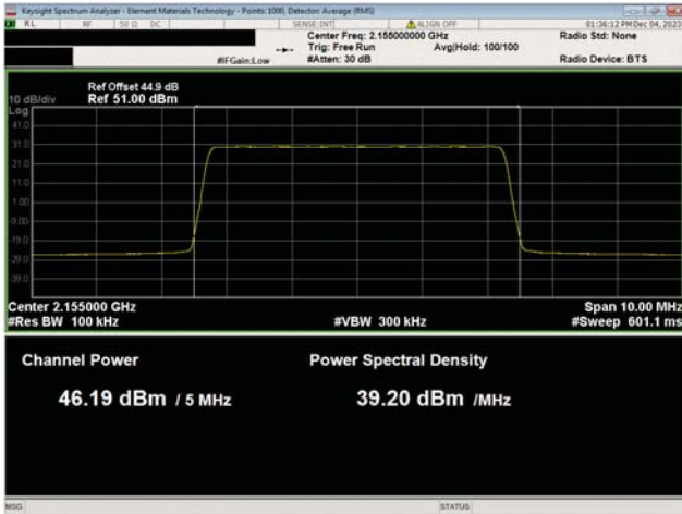
AWS Band n66, 2110 Mhz - 2200 MHz 5 MHz Bandwidth 64QAM Modulation Mid Ch, 2155.0 MHz
