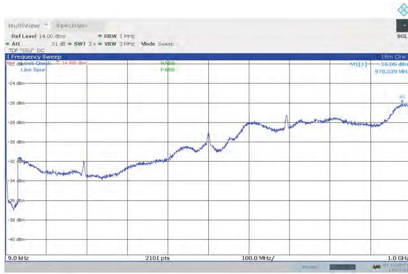
Spurious Emissions (9kHz - 1GHz) - QPSK (1962.5 MHz) (Band 25 NB-IoT IB 5MHz Channel BW)
