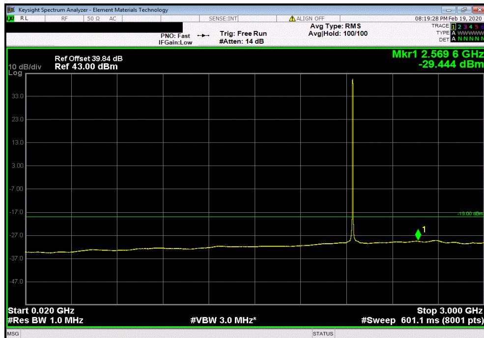
5G Band 66a 2110 MHz - 2180 MHz, (Single Carrier) Port 4, Mid Channel 2145 MHz, 5 MHz Bandwidth, 256-QAM Modulation, Range 4, 3 GHz - 6 GHz
