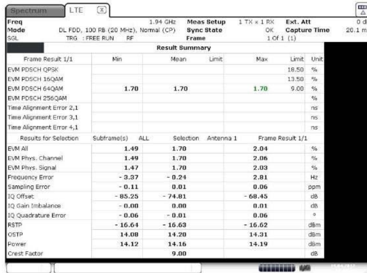
Figure 10 I/Q constellation table with I/Q error – 64QAM (1940.0 MHz) (20MHz Channel BW)
