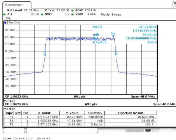
Figure 22 Occupied Bandwidth – 16QAM (1962.5 MHz) (20MHz Channel BW)
