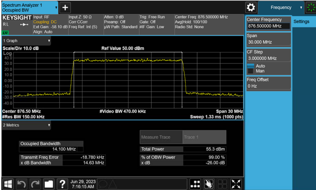
Channel Frequency 876.5MHz, 64QAM 15MHz BW, TX0
