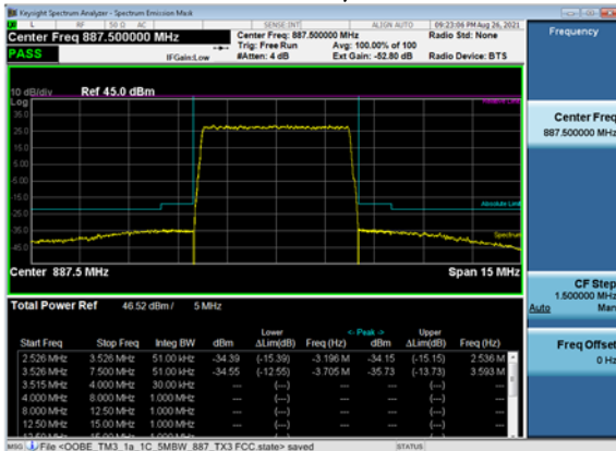
Channel Frequency 887.5MHz, 1C, 256QAM 5MHz BW, TX3
