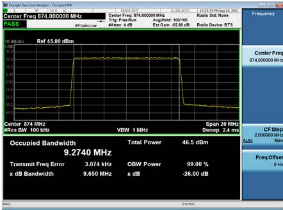
Channel Frequency 874MHz, 1C, 64QAM 10MHz BW, TX3
