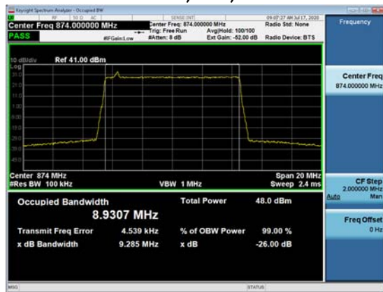
Channel Frequency 874MHz, 1C, QPSK 10MHz BW, TX1, Inband
