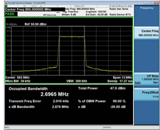
Channel Frequency 885MHz, 1C, 64QAM 3MHz BW, TX1
