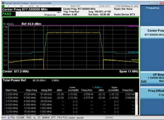
Channel Frequency 877.5MHz, 1C, 256QAM 5MHz BW, TX3
