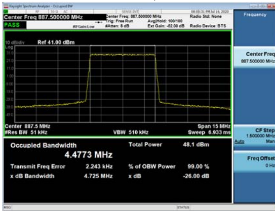
Channel Frequency 887MHz, 1C, QPSK 5MHz BW, TX1
