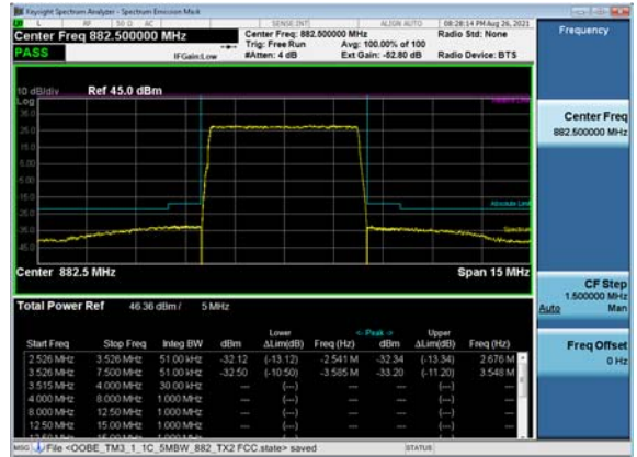
Channel Frequency 882.5MHz, 1C, 64QAM 5MHz BW, TX2
