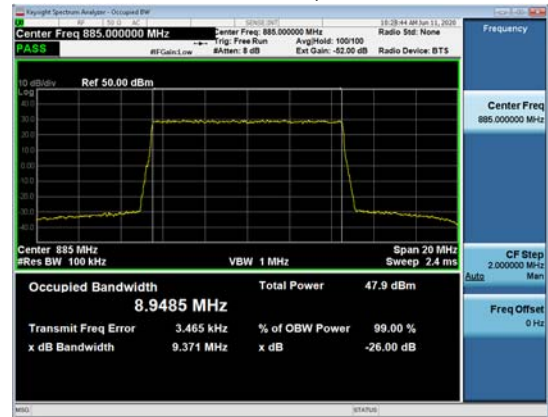
Channel Frequency 885MHz, 1C, 256QAM 10MHz BW, TX1
