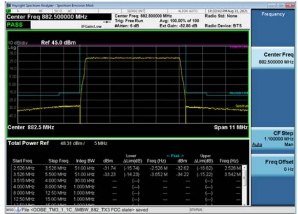
Channel Frequency 882.5MHz, 1C, 64QAM 5MHz BW, TX3
