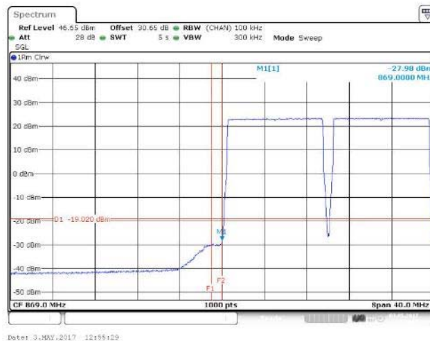
Figure 420 Spurious Emissions (Lower Band Edge) – QPSK (874 MHz, 884, 2 X 5 MHz Channel BW)
