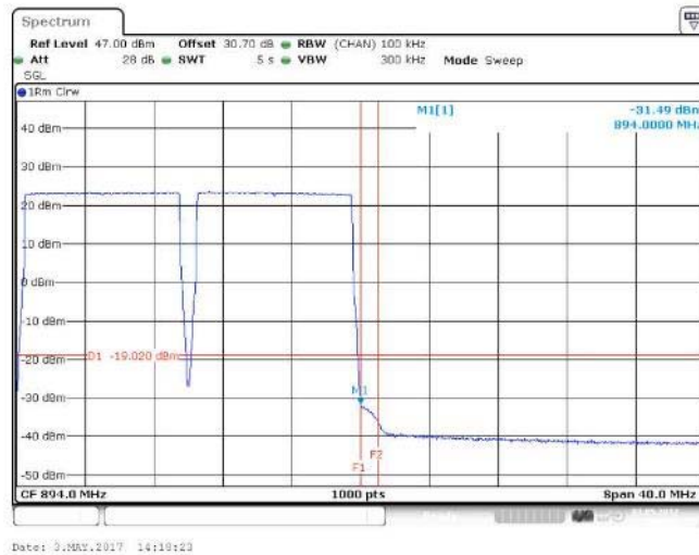
Figure 421 Spurious Emissions (Upper Band Edge) – QPSK (879,0 MHz, 889,0 MHz, 2 X 5 MHz Channel BW)
