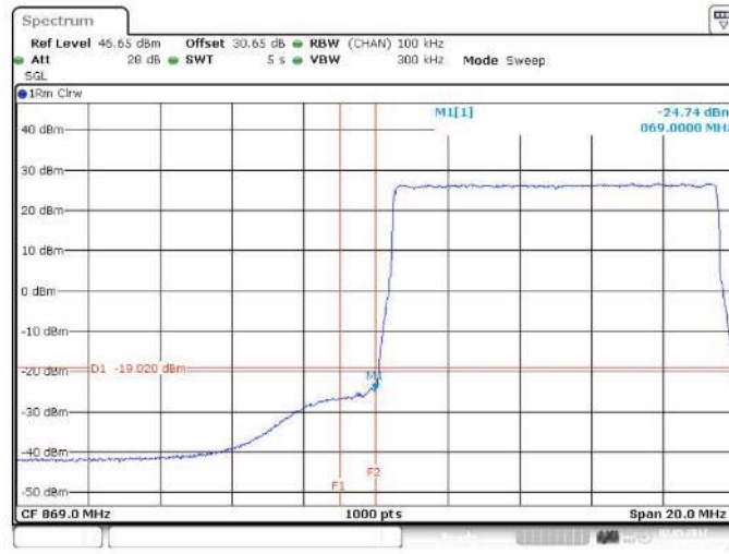
Figure 352 Spurious Emissions (Lower Band Edge) – 256QAM (874.0 MHz, 5 MHz Channel BW)
