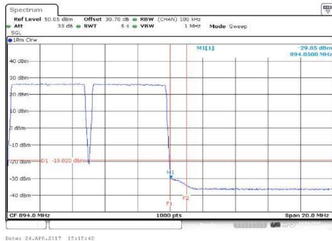
Figure 245 Spurious Emissions (Upper Band Edge) – QPSK (886.5 MHz, 891.5 MHz, 2 X 5 MHz Channel BW)
