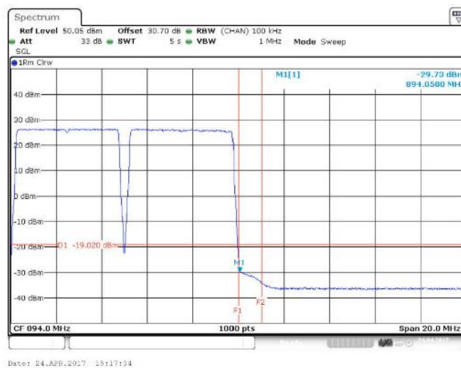
Figure 253 Spurious Emissions (Upper Band Edge) – 64QAM (886.5 MHz, 891.5 MHz, 2 X 5 MHz Channel BW)
