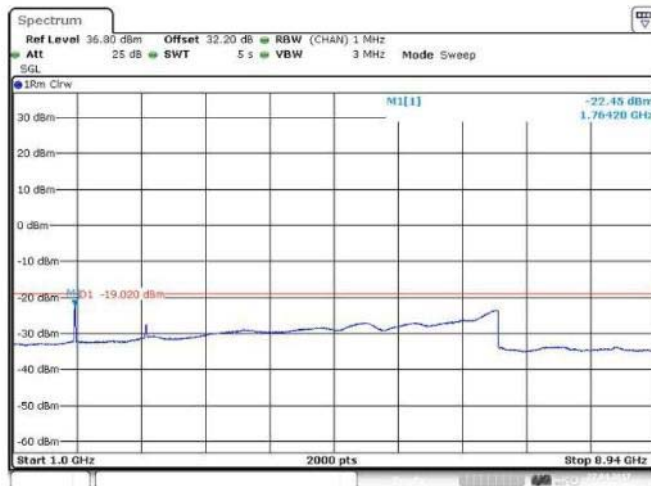
Figure 307 Spurious Emissions (1 GHz – 8.94 GHz) – 256QAM (876.5 MHz, 881.5 MHz, 886.5 MHz, 3 X 5 MHz Channel BW)
