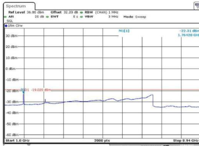
Figure 319 Spurious Emissions (1 GHz – 8.94 GHz) 64QAM (876.5 MHz, 881.5 MHz, 886.5 MHz, 3 X 5 MHz Channel BW)
