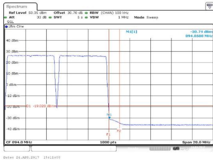
Figure 241 Spurious Emissions (Upper Band Edge) – 256QAM (886.5 MHz, 891.5 MHz, 2 X 5 MHz Channel BW)
