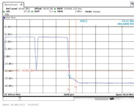
Figure 198 Spurious Emissions (Upper Band Edge) – QPSK (886.5 MHz, 891.5 MHz, 2 X 5 MHz Channel BW)
