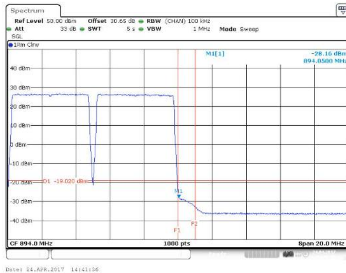
Figure 210 Spurious Emissions (Upper Band Edge) – 256QAM (886.5 MHz, 891.5 MHz, 2 X 5 MHz Channel BW)
