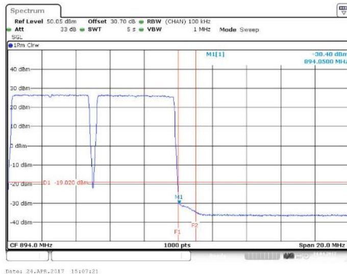
Figure 237 Spurious Emissions (Upper Band Edge) – 64QAM (886.5 MHz, 891.5 MHz, 2 X 5 MHz Channel BW)
