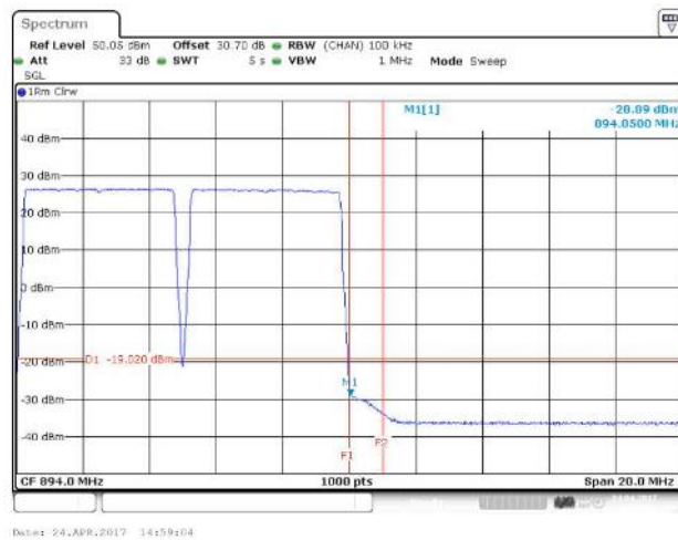
Figure 214 Spurious Emissions (Upper Band Edge) – QPSK (886.5 MHz, 891.5 MHz, 2 X 5 MHz Channel BW)
