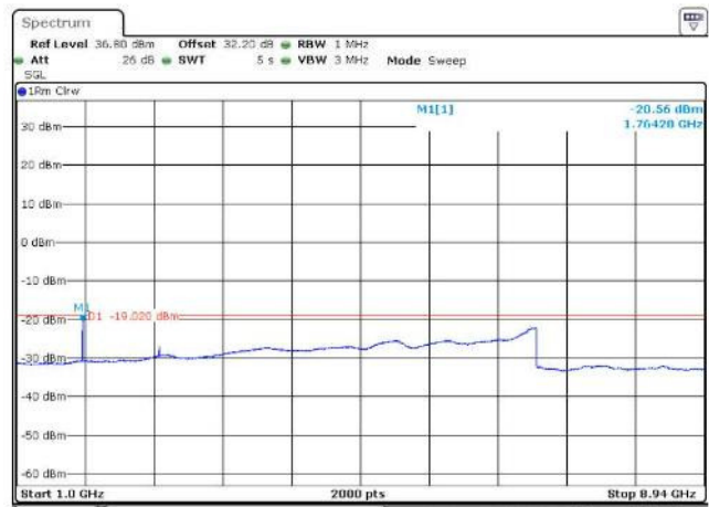
Figure 156 Spurious Emissions (1 GHz – 8.94 GHz) – 16QAM (881.5 MHz, 5 MHz Channel BW)
