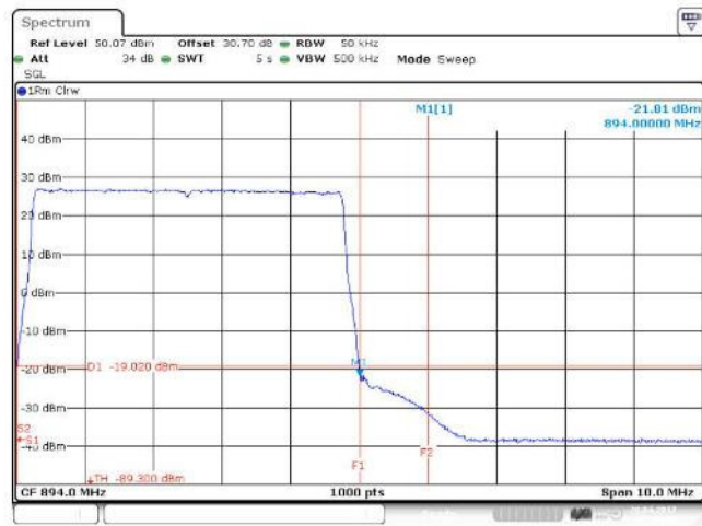
Figure 162 Spurious Emissions (Upper Band Edge) – 256QAM (891.5 MHz, 5 MHz Channel BW)
