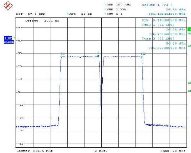
Figure 107 Occupied Bandwidth – 64QAM (879/884 MHz) (5+5MHz Channel BW)
