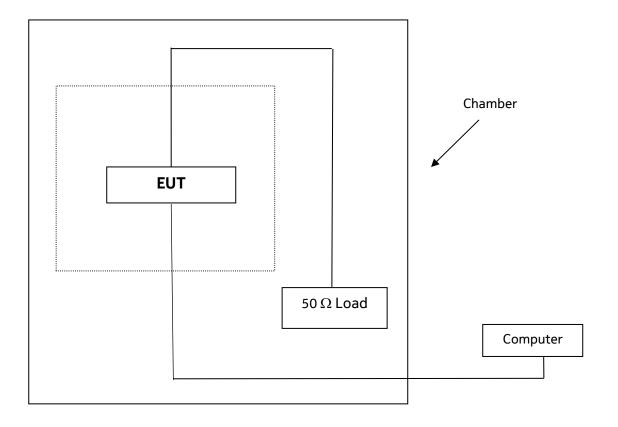
Figure 2. Setup Diagram of Radiated Test
