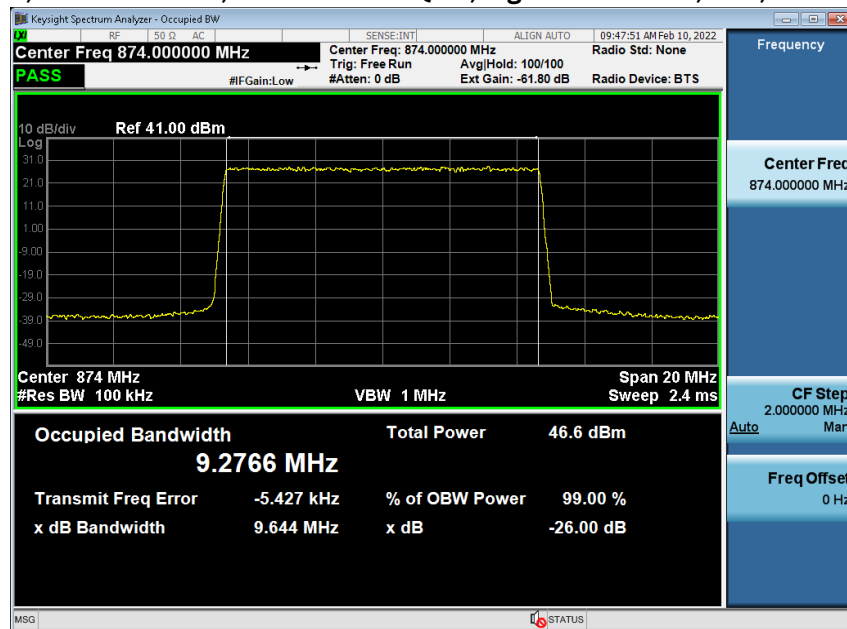
1C, Test Model 3.1, Modulation 64QAM, Signal BW 10MHz, TX4, 874MHz
