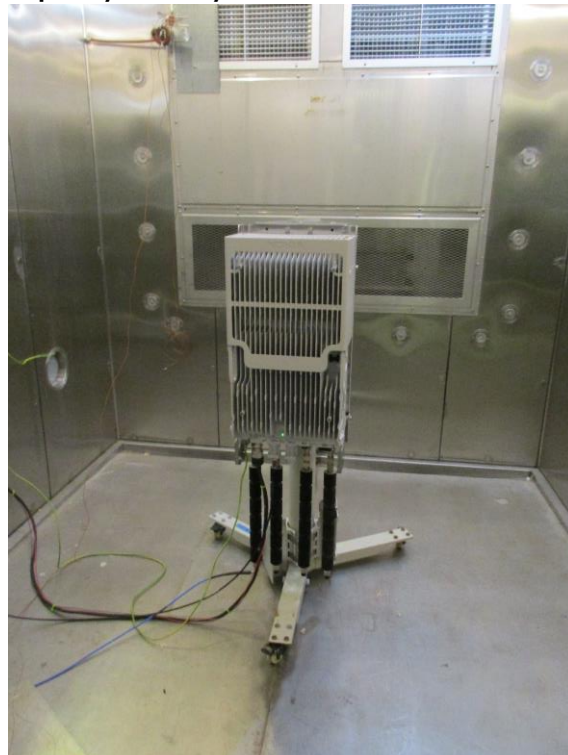
Frequency Stability – AHBCD in Thermal Chamber
