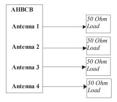
See ANSI C63.26-2015 paragraph 5.1 for details of test setup requirements. Based on antenna port conducted spurious emissions tests results, preliminary scans for radiated spurious emissions were performed in 30MHz – 9GHz frequency range.
