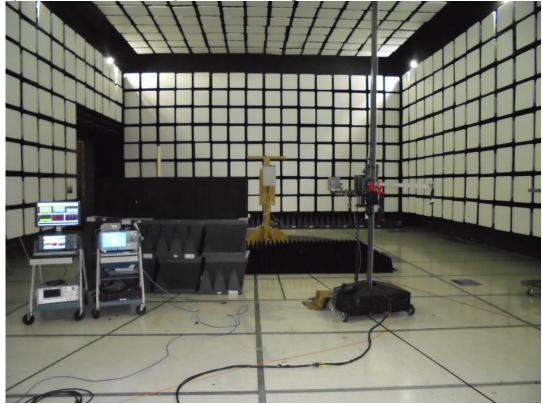
Radiated Spurious Setup for 40-100 GHz
