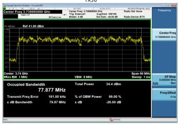
Test Model 3.2 Modulation QPSK/16QAM Channel Frequency 3840 + 3859.99 MHz TX36
