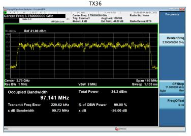
Test Model 3.2 Modulation QPSK/16QAM Channel Frequency 3840 + 3889.99 MHz
