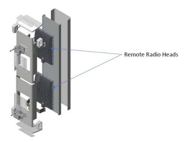
Each radio contains 16 transmitters. Each transmitter in the AAIB and AAFB is rated at 6.25W, and in the AAIC each transmitter is rated at 9.375W. Each radio will consist of a chassis, spine card, baseband/RF boards, filter, and antenna, stacked as shown below.
