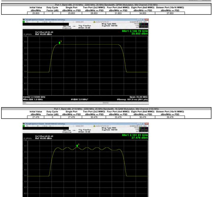
Span 35.00 MHz #Sweep 601.0 ms (601 pts)
