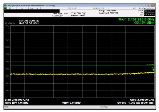
Band 66 (Single Carrier) Port 2, 20 MHz, NB-IoT, High Channel, 2190 MHz, High Channel Range 1 (2.19 GHz - 2.201 GHz)
