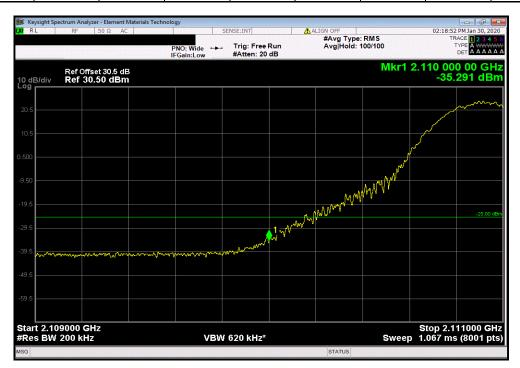
Band 66 (Single Carrier) Port 2, 20 MHz, NB-IoT, Low Channel, 2120 MHz, Low Channel Range 2 (2.109 GHz - 2.108 GHz)
