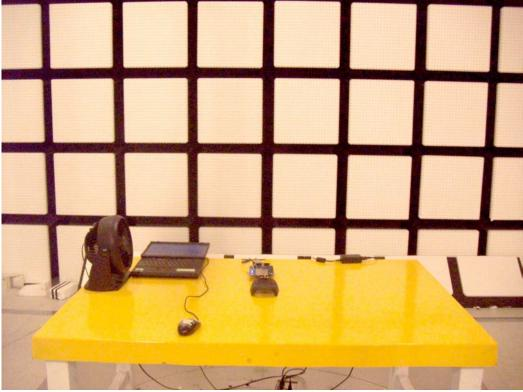
NOTE: EUT placed in worst-case orientation for emissions (X-orientation)
