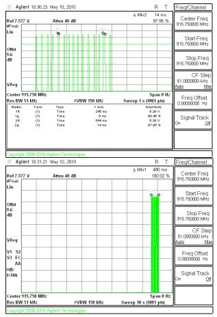
7.1 msec/pulse x 16 pulses/490 msec burst = 113.6 msec in 10 seconds total Meets 0.4 second occupancy/10 seconds limit.
