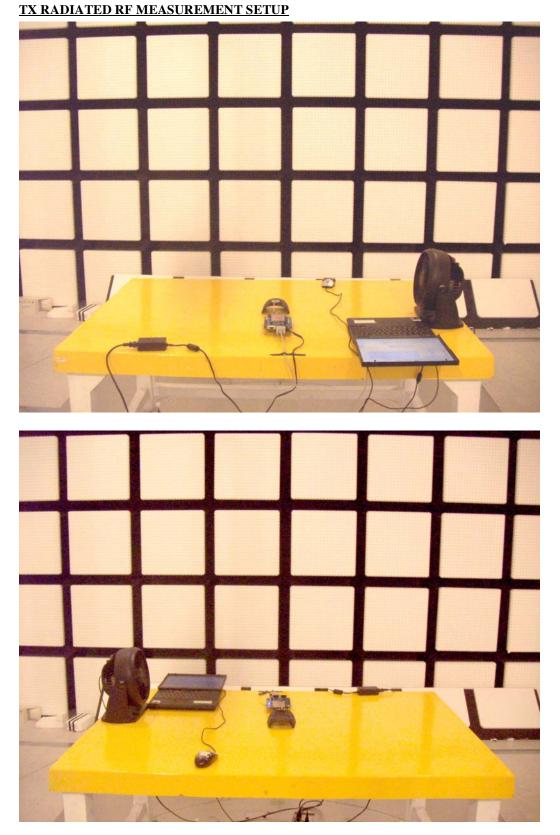
NOTE: EUT placed in worst-case orientation for emissions (X-orientation)
