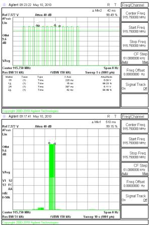
16 msec/pulse x 11 pulses/burst + 42 msec pulse = 218 msec total in 10 seconds Meets 0.4 second occupancy/10 seconds limit.
