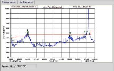
Note: Emissions over class B limit line are from test fixture or are TX emissions more than -20dBc below fundamental
