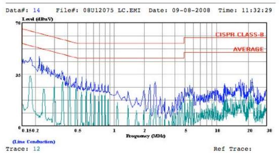
Condition: CISPR CLASS-B Test Operator:: Tom Chen Project #: : 08U12075 Company: : Intelleflex Configuration:: EUT with peripherals Mode: : Transmit Normal Target: : FCC Class B Voltage: : 115 VAC / 60 Hz : L2: Peak (Blue); Average (Green) : RFID Reader FCC ID:UBLIB500
