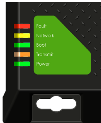
Figure 2.3-3 LED Activity and Status Lights
