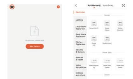
**Step 2** Select "Electrician". Power the device on and make sure the blue indicator is flashing quickly. If you do not see a flashing blue light press and hold the reset button for 5 seconds.
