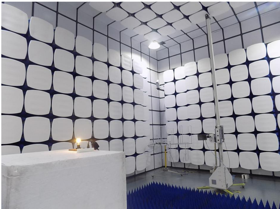
2.Setup for Radiated Emission above 1GHz
