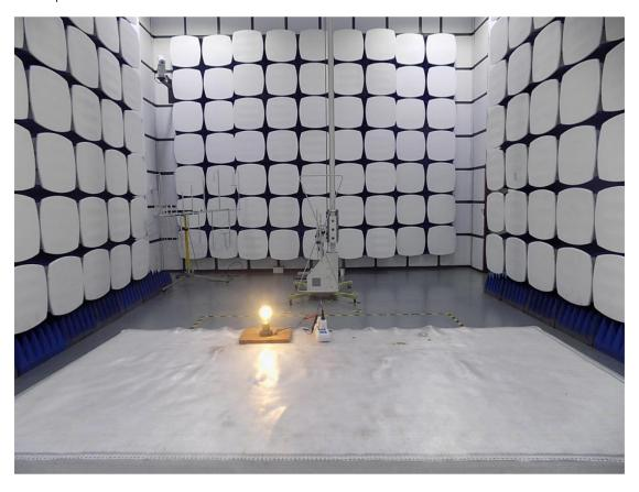
2.Setup for Radiated Emission above 1GHz
