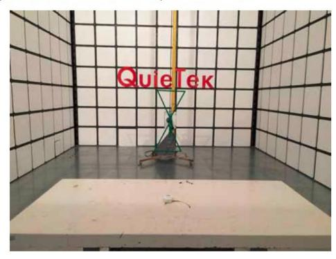
Description: Radiated Emission Test Setup for 1~18GHz
