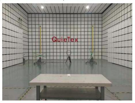
Description: Radiated Emission Test Setup for 30MHz~1GHz
