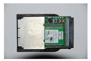
Internal view of device showing open core antenna and rear of PCB.
