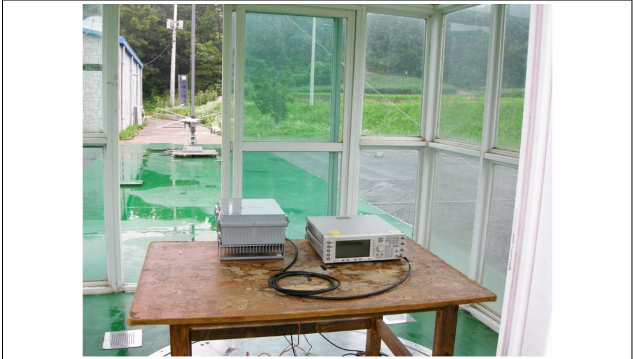
Figure 3 Test setup for Radiated Emissions
