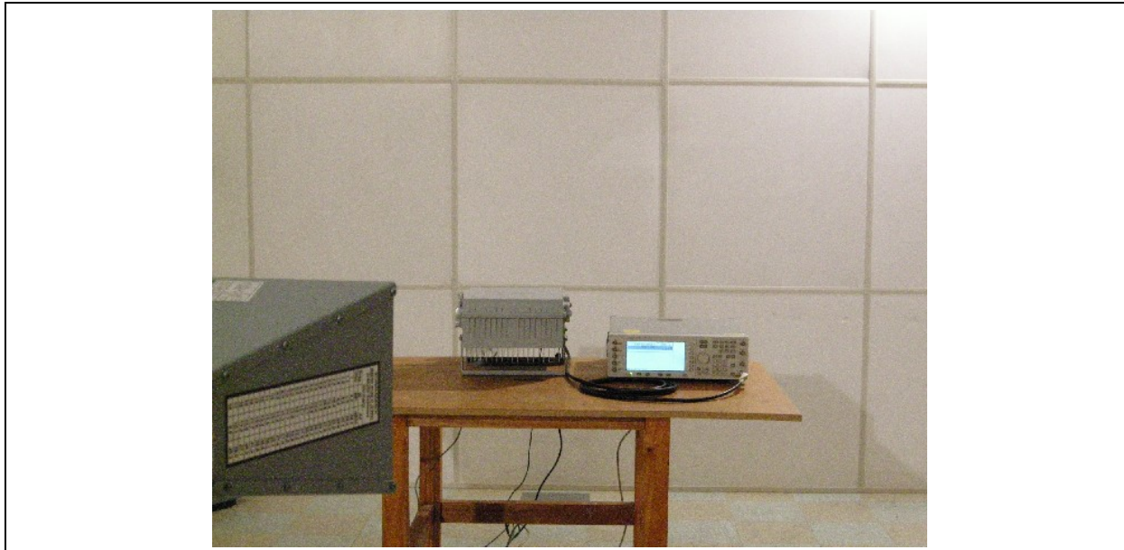
Figure 8 Test setup for Spurious Radiated Emissions
