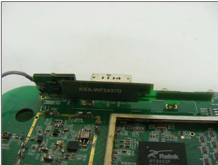
WALN Antenna view
