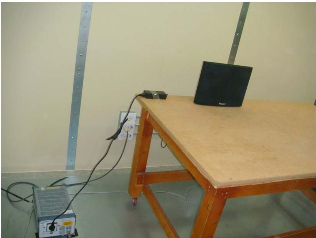
**<AC Power Line Conducted Emissions - Rear View>**
