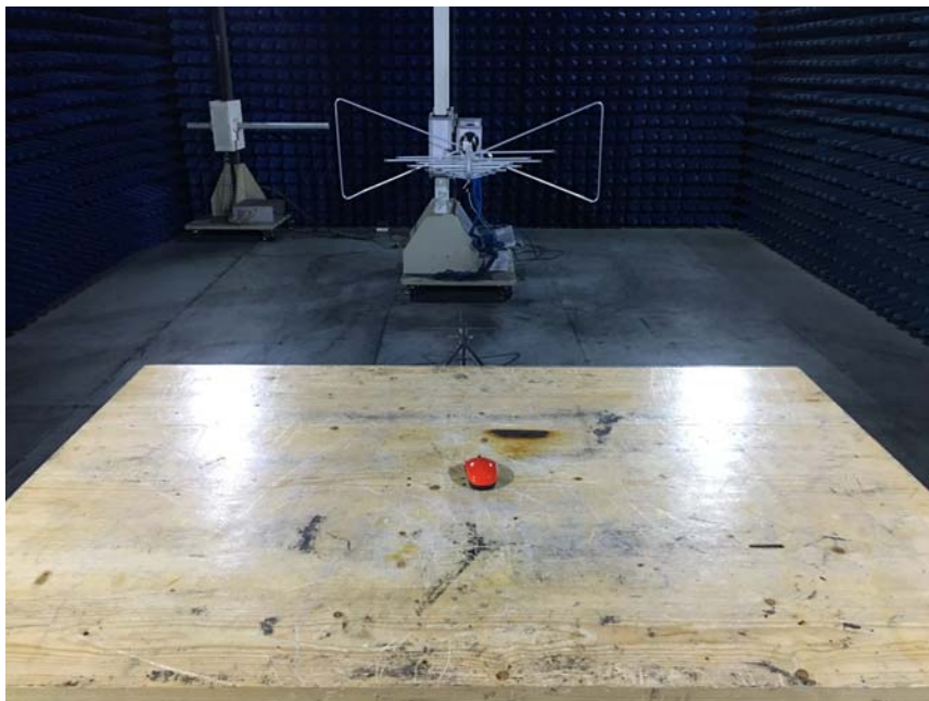
Photograph of set-up for Radiated Emission below 1000MHz
