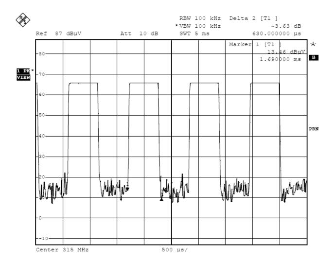
The graph show the duration of short 'on' signal. From marker 1 to marker 2, duration is 0.63ms.
