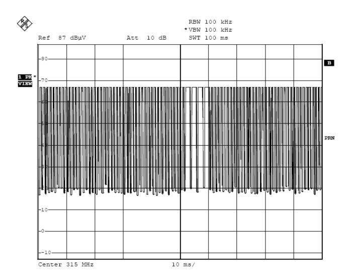
The graph shows the pattern of coding during the signal transmission. It sums of 4 long 'on' signals and 82 short 'on' signals.
