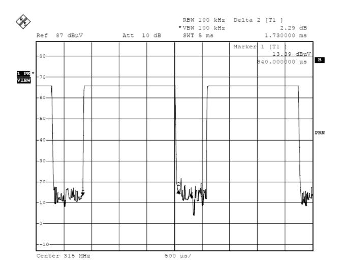
The graph show the duration of long 'on' signal. From marker 1 to marker 2, duration is 1.73ms.
