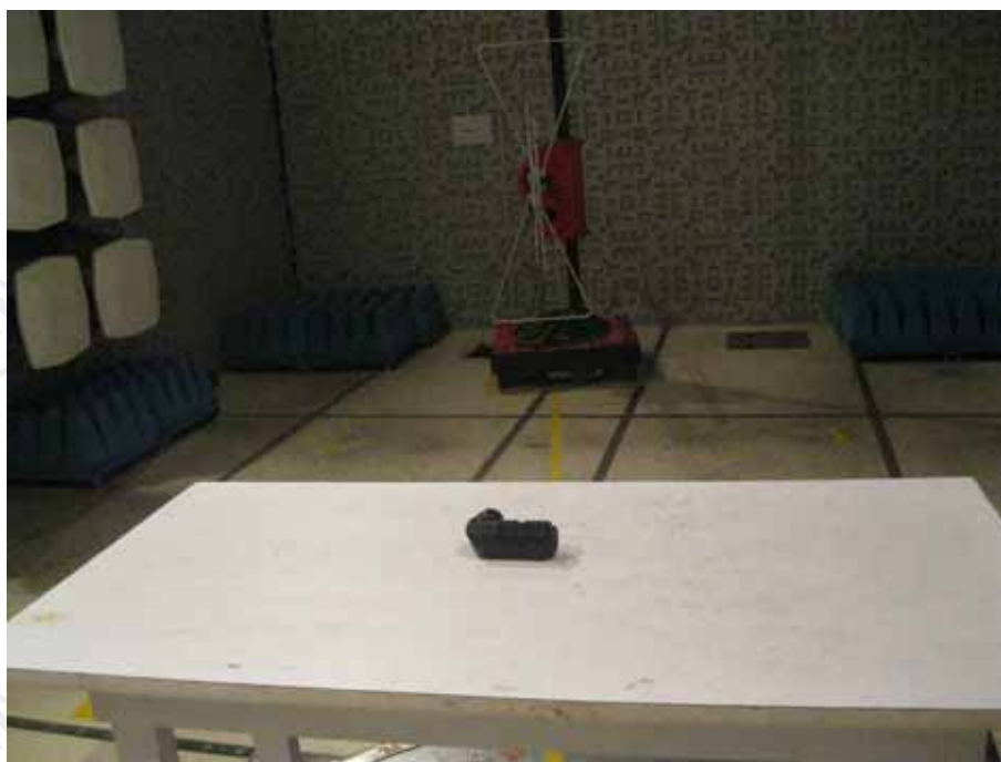
TEST SETUP OF RADIATED EMISSION (30MHz ~ 1GHz)
