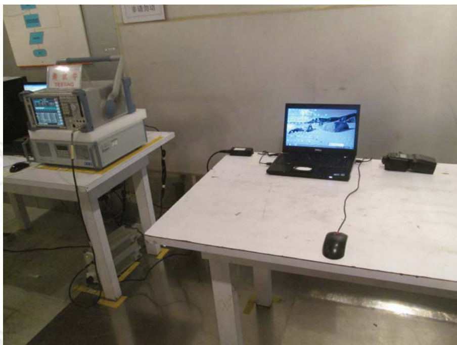
TEST SETUP OF CONDUCTED EMISSION
