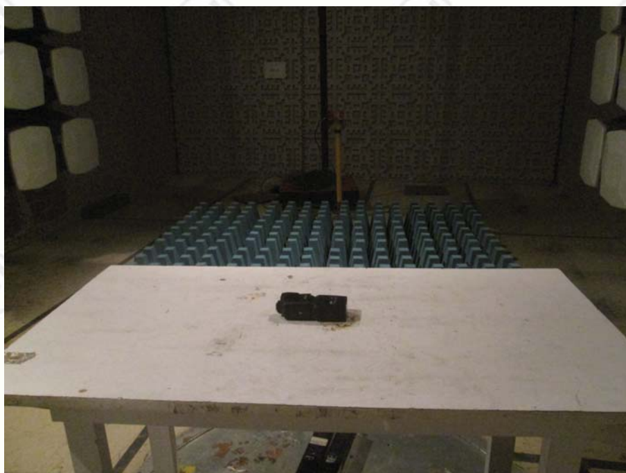
TEST SETUP OF RADIATED EMISSION (Above1GHz)
