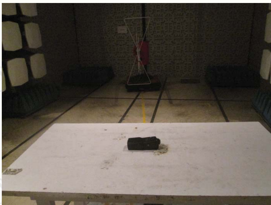
TEST SETUP OF RADIATED EMISSION (30MHz~1GHz)
