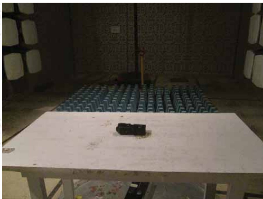
TEST SETUP OF RADIATED EMISSION (Above1GHz)
