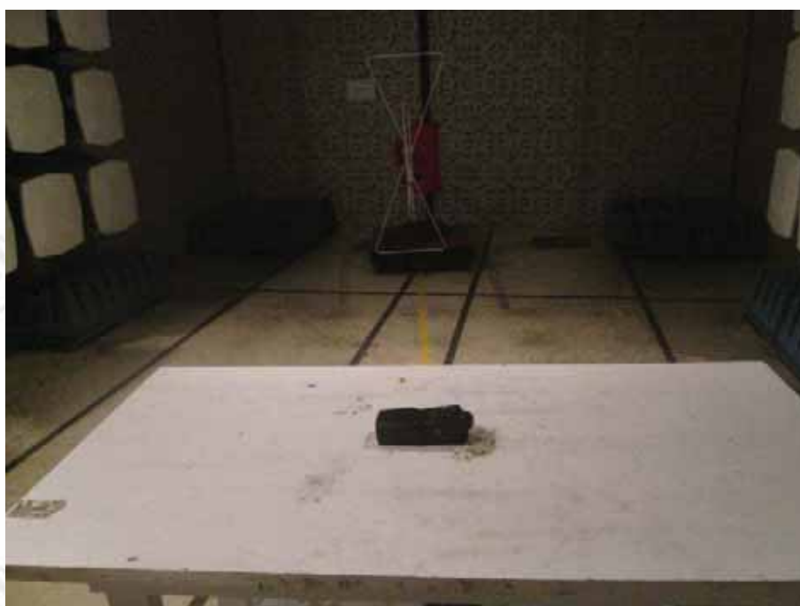
TEST SETUP OF RADIATED EMISSION (30MHz~1GHz)
