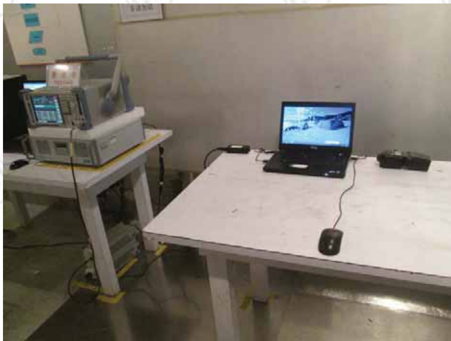
TEST SETUP OF CONDUCTED EMISSION
