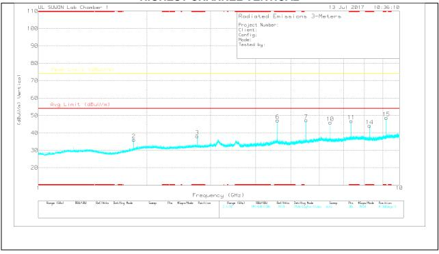
Note: Emission was scanned up to 10 GHz
