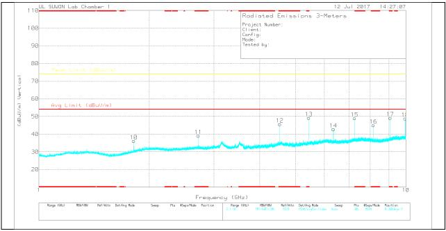
Note: Emission was scanned up to 10 GHz
