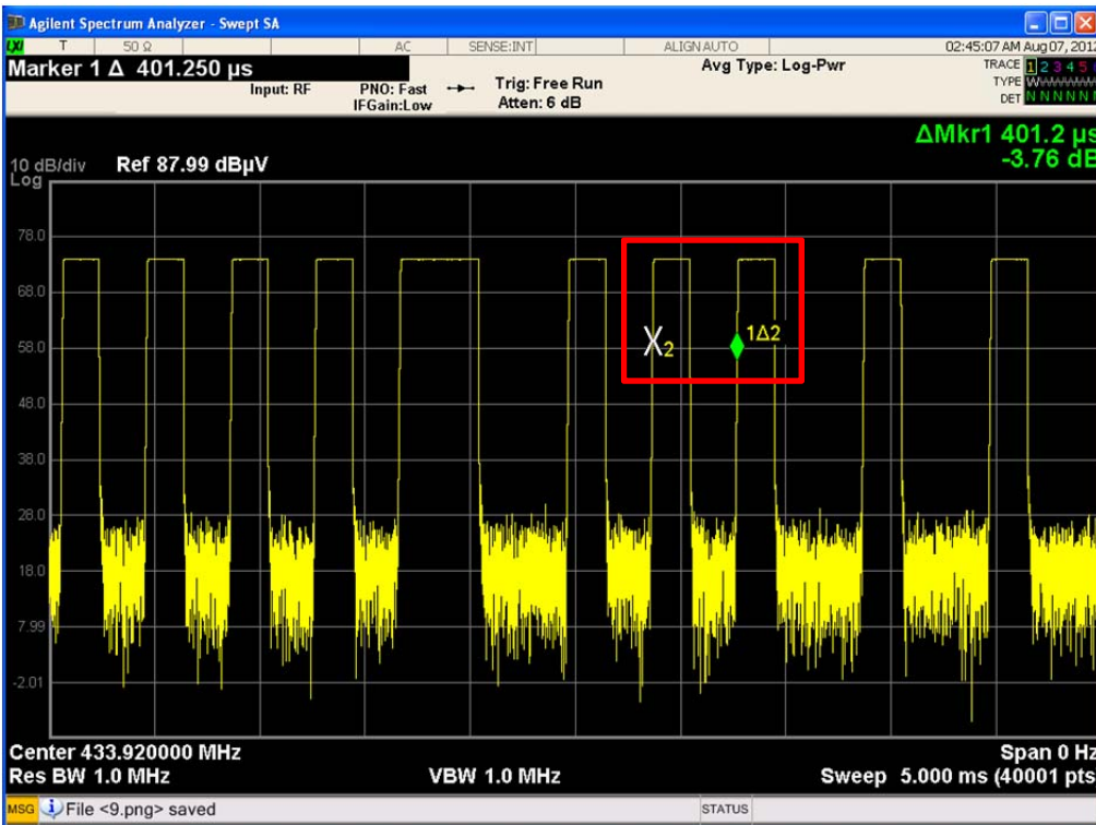
Period of Type 2 (Bit 0) : 401.2 μs
