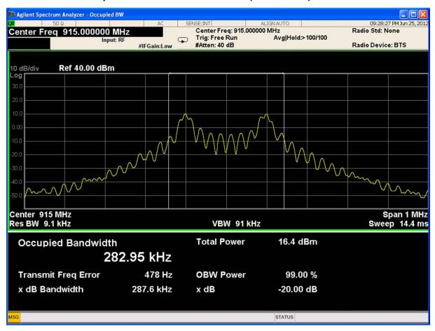
20 dB Bandwidth: 287.6 kHz99 % Bandwidth: 282.95 kHz
